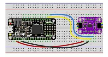
Board 3V to sensor VIN (red wire) Board GND to sensor GND (black wire) Board SCL to sensor SCL (yellow wire) Board SDA to sensor SDA (blue wire)
