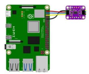
Pi 3V to sensor VIN (red wire) Pi GND to sensor GND (black wire) Pi SCL to sensor SCL (yellow wire) Pi SDA to sensor SDA (blue wire)
