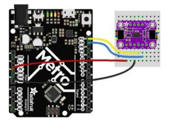
Board 5V to sensor VIN (red wire) Board GND to sensor GND (black wire) Board SCL to sensor SCL (yellow wire) Board SDA to sensor SDA (blue wire)
