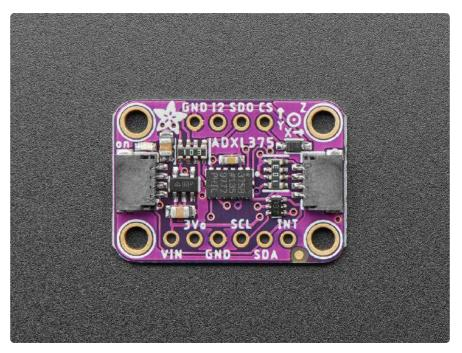
Hey rocket man (burnin' out your fuse out there alone) ever wonder how fast you're rocketing? The Adafruit ADXL375 High G Accelerometer is an epic +-200g 3-axis accelerometer may be able to tell the answer.
