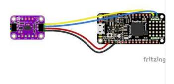
Board 3V to sensor VIN (red wire) Board GND to sensor GND (black wire) Board SCL to sensor SCL (yellow wire) Board SDA to sensor SDA (blue wire)
