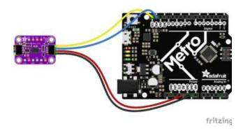
Board 5V to sensor VIN (red wire) Board GND to sensor GND (black wire) Board SCL to sensor SCL (yellow wire) Board SDA to sensor SDA (blue wire)
