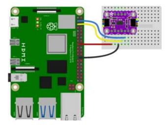
Pi 3V to sensor VIN (red wire) Pi GND to sensor GND (black wire) Pi SCL to sensor SCL (yellow wire) Pi SDA to sensor SDA (blue wire)
