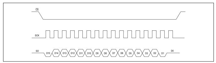
Figure 1a. Serial Interface Protocol
