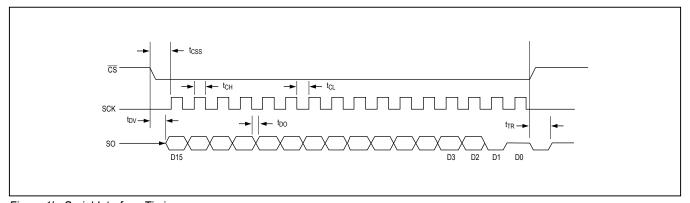
Figure 1b. Serial Interface Timing
