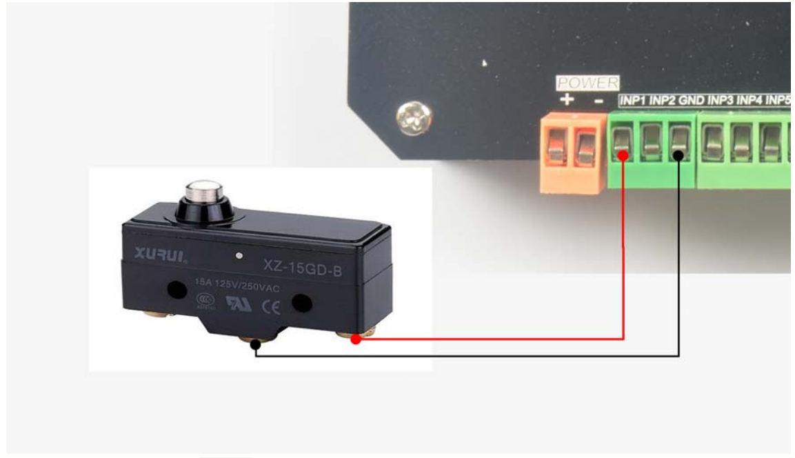
Figure2-4. Probe/Estop/ ordinary fretting switch input connection
