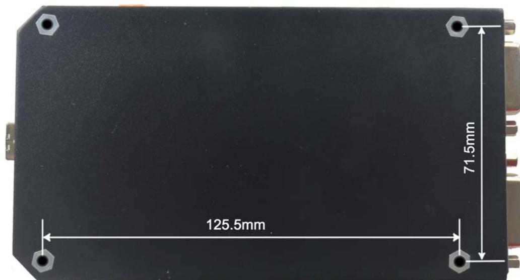
Figure1-2. The other side of NVCM and installation dimensions
