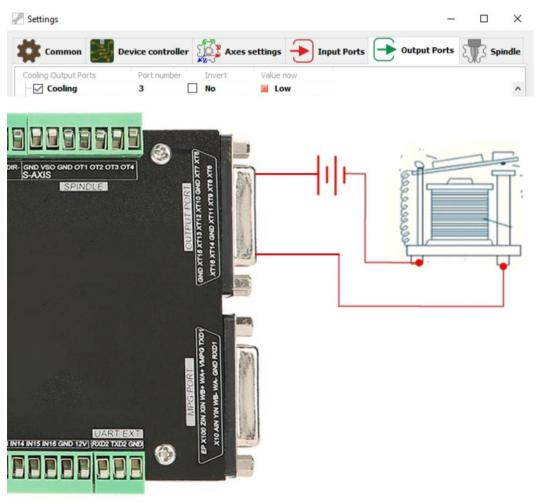
**7 -** Spindle control output. GND1 (Output GND), VSO (0-10V adjustable speed output), INDEX (spindle speed feedback input), OUT1 (common output port 1), OUT2 (common output port 2).
