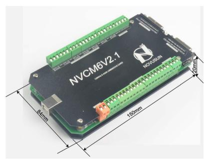
The bottom install size is 125.5mm\*71.5mm.
