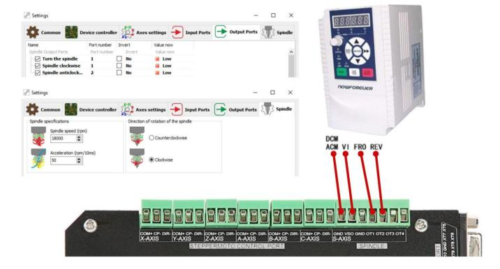
**8 -** Terminal block is 6 axis stepper driver control output interface, from left to right, there are X,Y,Z,A,B,C 6 axis output, it's common anode, the cable connection for each axis is COM+/CP-/DIR-, COM is common+ ,CP is Pulse-, DIR is direction-.
