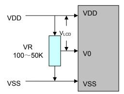
We recommend allowing field adjustment of V0 for all designs. The optimal value for V0 will change with temperature, variations in VDD, and viewing angle. V0 will also vary module-to-module and batch-to-batch due to normal manufacturing variations.
