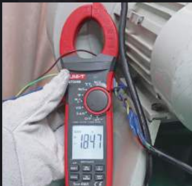
Inrush current capture (UT206B/207B/208B)
