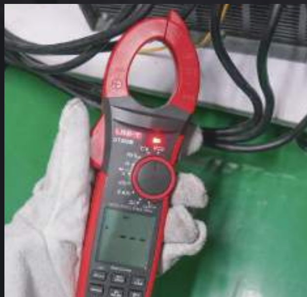
NCV Multi-Segment Display and audio/visual alarm
