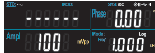
Picture 4-17 Set frequency sweep waveform
