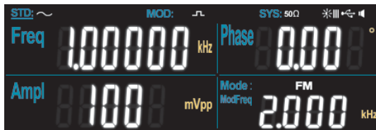
Picture 4-13 Set FM carrier waveform
