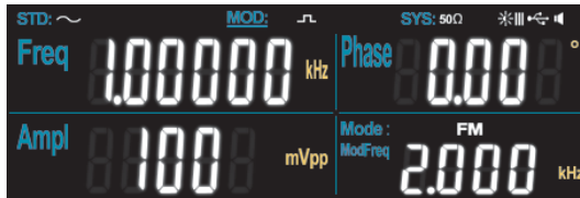
Picture 4-12 Set FM modulation frequency and waveform
