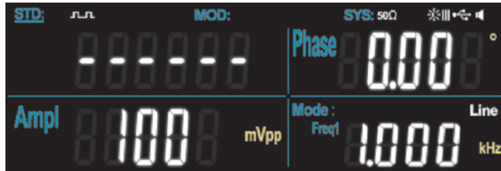
Picture 4-20 Set frequency sweep waveform
