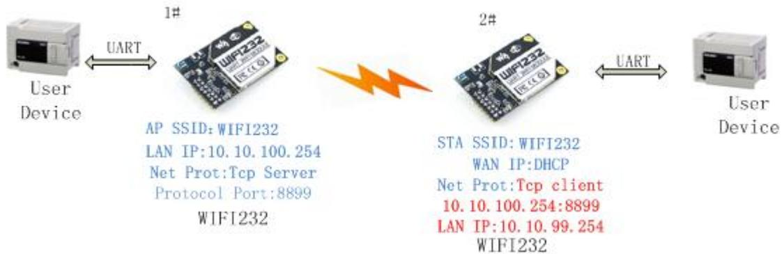
Figure 49 Transparent Serial Port Application
