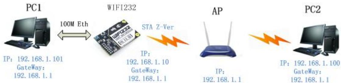
Figure 22 **WIFI232 Ethernet Interface Networking (As STA, Z-Ver)**
