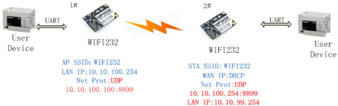
Figure 54 Configure Transparent Serial Port Connection (UDP)
