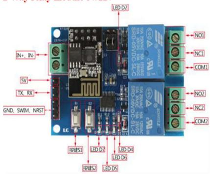
IN +, IN-: 5V / 12V power input; TX, RX: UART serial port pins;
