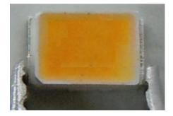
(3) When populating boards in SMT production, there are basically no restrictions regarding the form of the pick and place nozzle, except that mechanical pressure on the surface of the resin must be prevented. This is assured by choosing a pick and place nozzle which is larger than the LED's reflector area.
