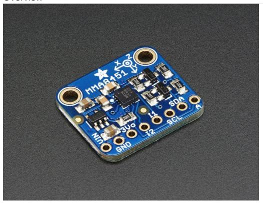
You can detect motion, tilt and basic orientation with a digital accelerometer - and the MMA8451 is a great accelerometer to start with. It's low cost, but high precision with 14-bit ADC. It has a wide usage range, from +-2g up to +-8g yet is easy to use with Arduino or another microcontroller
