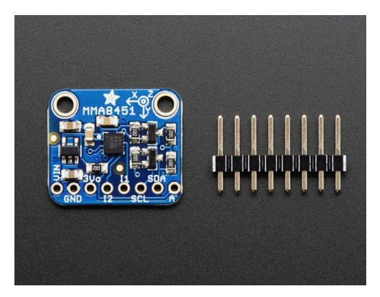
This sensor communicates over I2C so you can share it with a bunch of other sensors on the same two I2C pins. There's an address selection pin so you can have accelerometers share an I2C bus. Please note this chip requires repeated-start I2C support (in case you are looking to port this to another processor)
