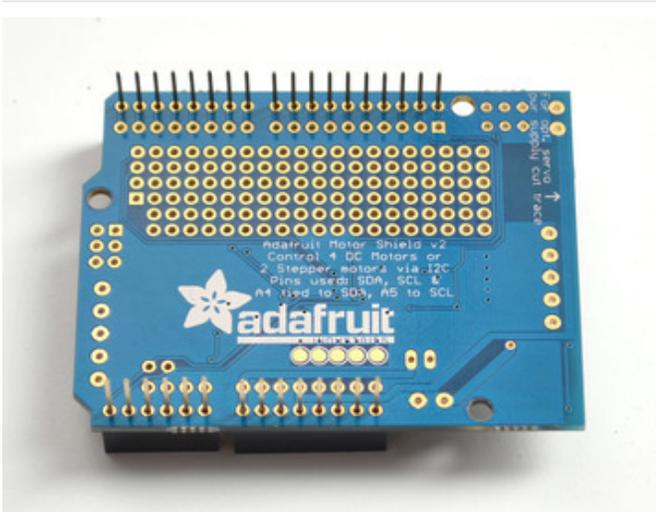
Start by sliding the 10 pin, 2 x 8 pin and 6-pin stacking headers into the outer rows of the shield from the top. Then flip the board over so its resting on the four headers. Pull on the legs if necessary to straighten them out.
