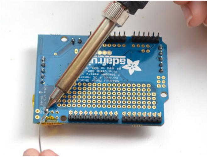
Then flip the board over and solder the 6 pins
