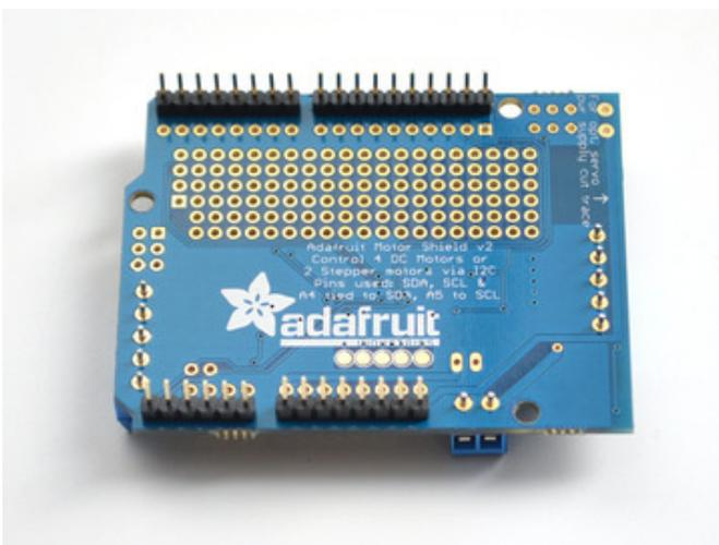
Flip the board over so that you can see & solder the pins of the terminal blocks
