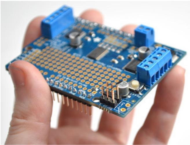
OK next up take the **2x3 pin header** and place it with the short legs down into the top corner where it says SERVO 1 and SERVO 2
