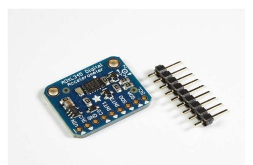
The board comes with all surface-mount components pre-soldered. The included header strip can be soldered on for convenient use on a breadboard or with 0.1" connectors. However, for applications subject to extreme accelerations, shock or vibration, locking connectors or direct soldering is advised.
