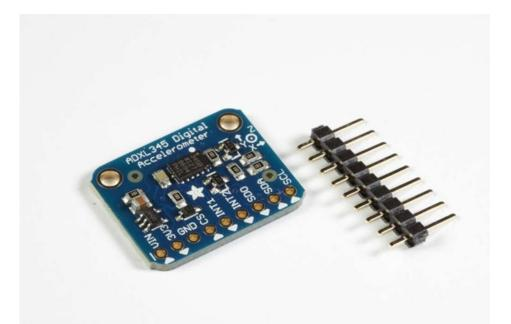
The ADXL345 is a low-power, 3-axis MEMS accelerometer modules with both I2C and SPI interfaces. The Adafruit Breakout boards for these modules feature on-board 3.3v voltage regulation and level shifting which makes them simple to interface with 5v microcontrollers such as the Arduino.
