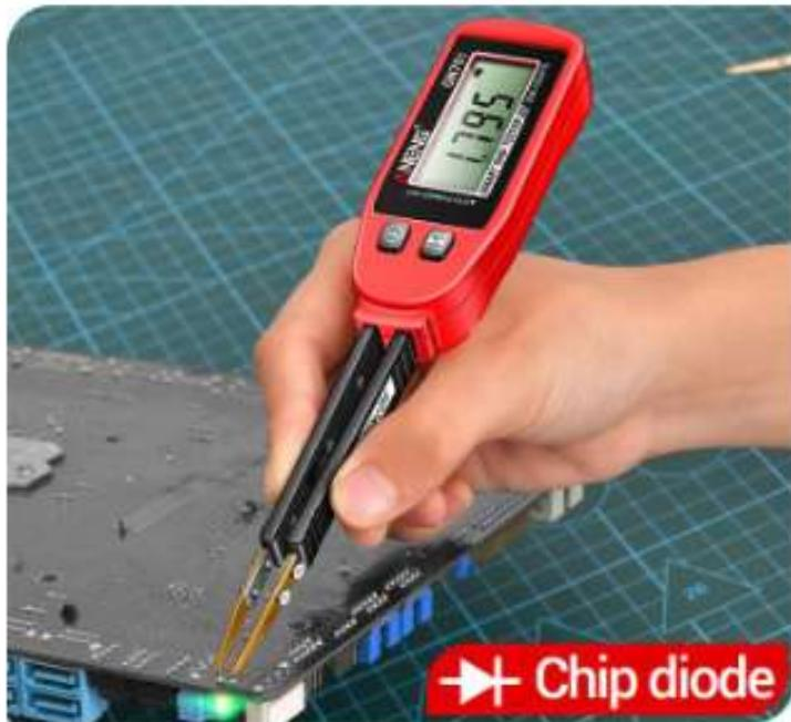
Instrument nib test end alignment diode positive and negative test.
