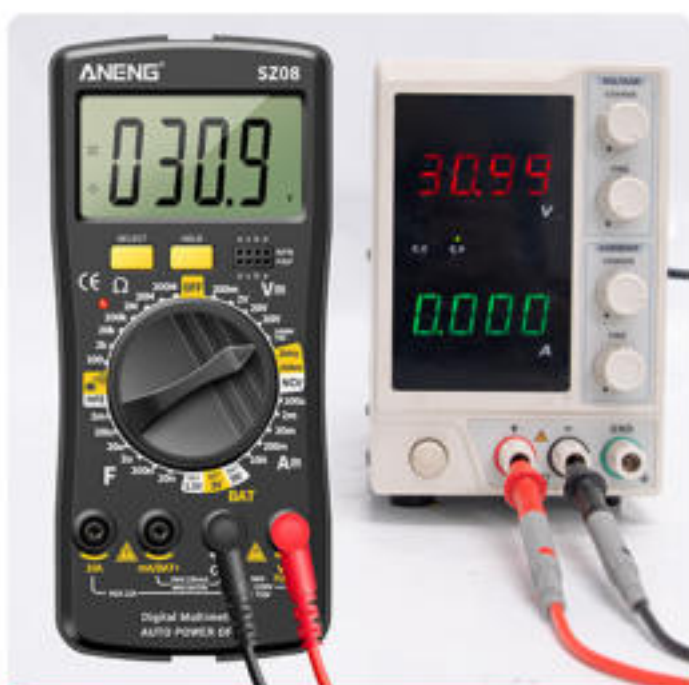
DC voltage measurement
