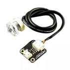
This is a photoelectric liquid level sensor that is operates using traditional optical principles. The advantages of this are a high sensitivity and no need for mechanical parts - meaning less calibration! The corrosion resistant probe is easily mounted and can handle high temperatures and high pressures. The sensor is equipped with an interface adapter for compatibility with the DFRobot "Gravity" interface.
