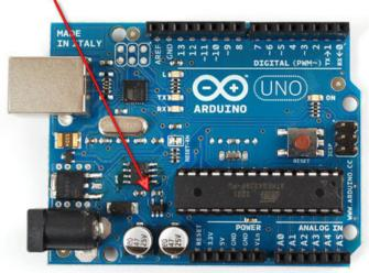
One sad thing about older boards is that they had a 3.3v power supply but it was really just whatever the FTDI chip's internal 3.3v regulator could give. You -could- get 50mA out of it, maybe. But high power stuff like XBees, SD cards, some fast ADC or DACs could easily drag down the FTDI chip and reset the USB connection. The Uno solves this problem by adding a new 3.3V regulator the LP2985 which can easily provide 150mA.
