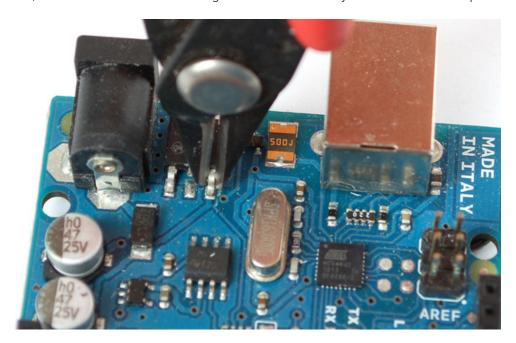
Then you'll need to heat the tab up to get it liquid so you can lift off the old part. Although it may seem counter intuitive, its best to **add** some solder to the tab, melt it on with your iron, this will improve the heat conduction since the tab is so large.
