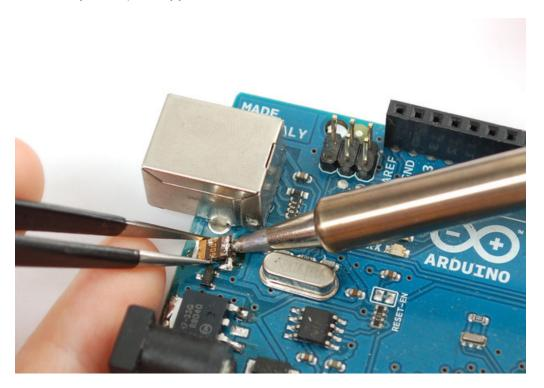
Clip the diode short and bend the leads over. Solder the side without a stripe (anode) to the old fuse pad, nearest the board edge. Solder the striped end (cathode) to the right hand leg of the regulator.
