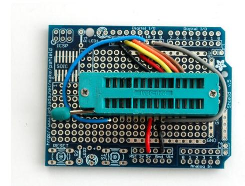
Follow the protoshield tutorial to solder in the Red LED into **LED1** position, Green LED into **LED2** position. Also solder in the two 1.0K resistors next to the LEDs. We'll use the LEDs as indicators. Then solder a wire from the LED2 breakout (white) to analog 0 and a wire from LED1 breakout (white) to digital 8.
