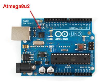
The Uno has changed that by exchanging the FT232RL chip with an atmega8u2 chip. There are a few things that are possible with this new chip but before we discuss that lets make it clear that by default, this chip acts identically to the FTDI chip that it replaces. It's just a USB-serial port!
