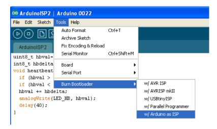
On newer versions of the Arduino IDE, select **Arduino as ISP** from the **Tools Programmer** menu, then select **Burn Bootloader** from the Tools menu.
