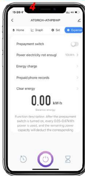
KWH consumption setting, when reaching the set value, it will alarm and shut down the device
