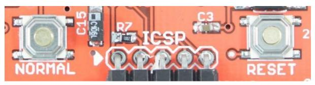
**New in Bus Pirate V4 are two buttons.** NORMAL starts the Bus Pirate without loading any settings saved in the EEPROM - useful if something when wrong. RESET simply resets the PIC.
