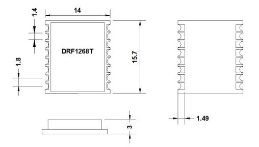
Figure 3: Mechanical Dimension
