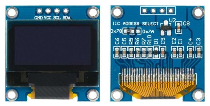
In contrast to LCD technology, Organic Light-Emitting Diode (OLED) displays do not require a backlight and are regarded as the ultimate technology for the next generation of flat-panel displays.
