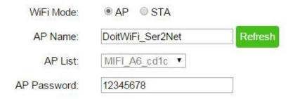
If STA mode is chosen, "refresh" and "AP List" buttons will be enabled. "Refresh" may be used to scan other WiFi signal, and the scanned result will be shown in the "AP List".
