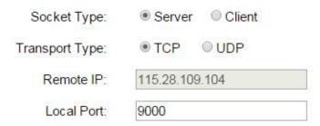
When "Client" mode is set, "Remote IP" is enabled. "Remote IP" and "Remote Port" should be filled in.
