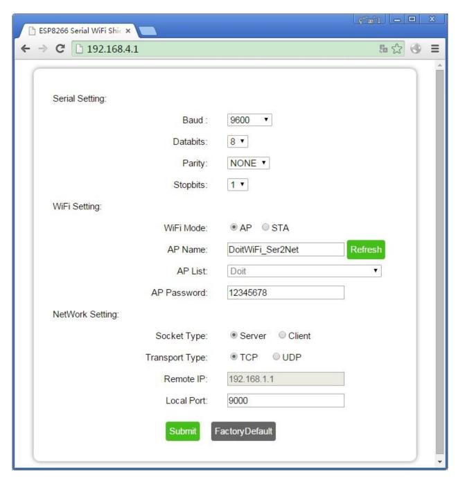
Built-in WebServer in the serial WiFi shield supports serial parameters configuration, network parameter configuration. And It also supports automatic or manual AP scan.
