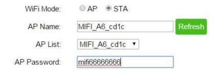
When the serial WiFi shield is in the STA mode, it will always try to connect the specified wireless router till the connection is built or configuration mode is set.
