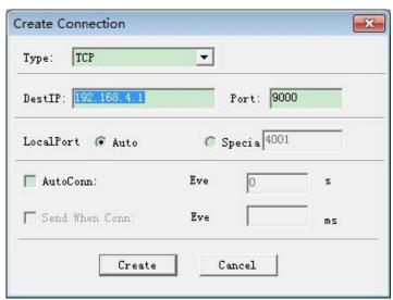
Once connection is build successfully, the software shows the transported data from serial WiFi shield every one second. Therefore, Arduino can send the serial data to the network.
