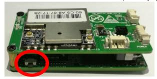
Step4: Waiting for the Transmitter blue LED turn on more then 10 seconds. That means the configuration have completed.
