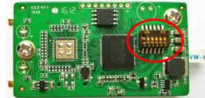
There are 6 group Dial-up in the module . ON direction is showing low-level ,marked as 0.
