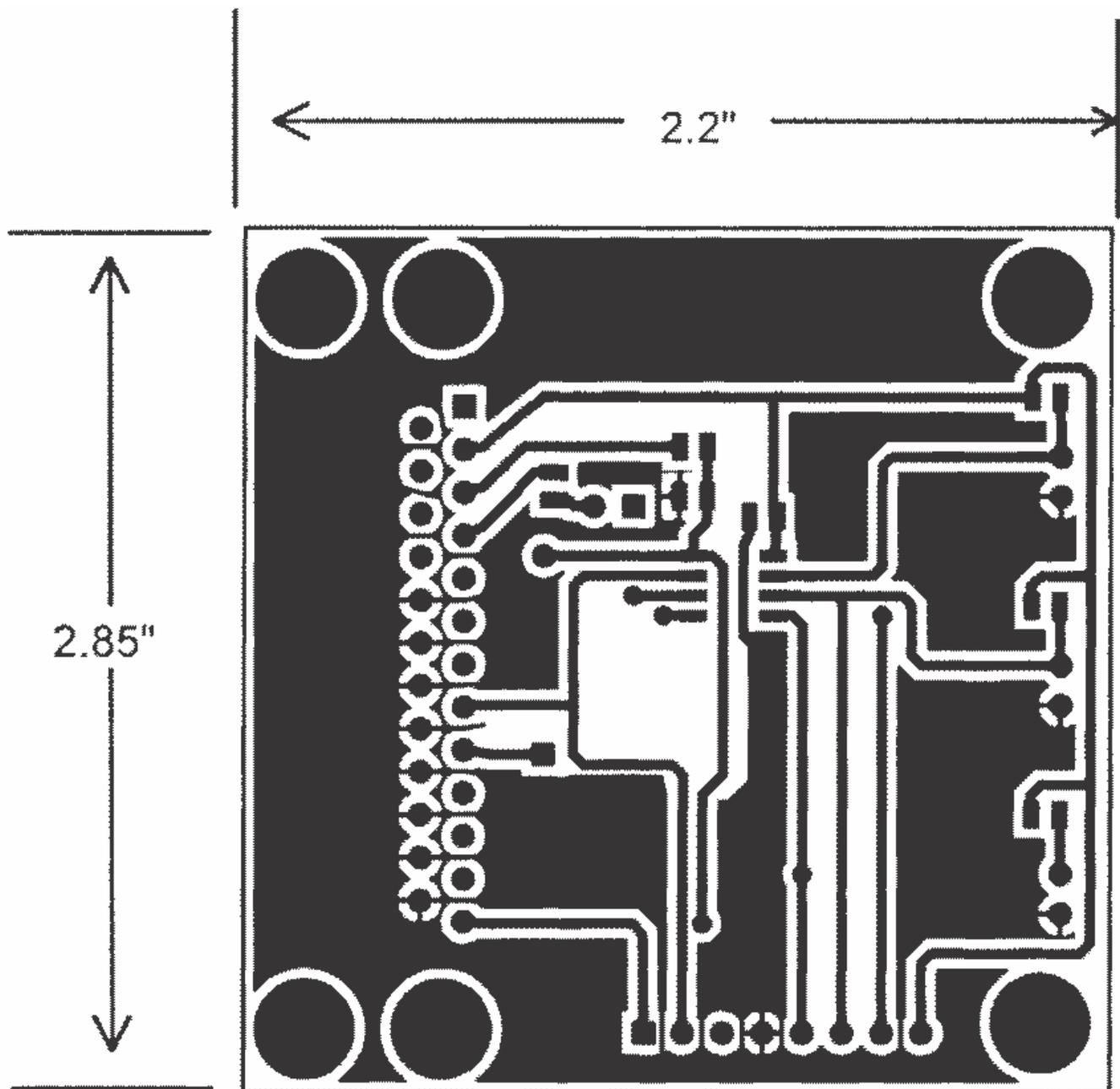
LM75C  $\theta_{JA}$  (thermal resistance, junction-to-ambient) when attached to a printed circuit board with 2 oz. foil similar to the one shown. Summarized below:
