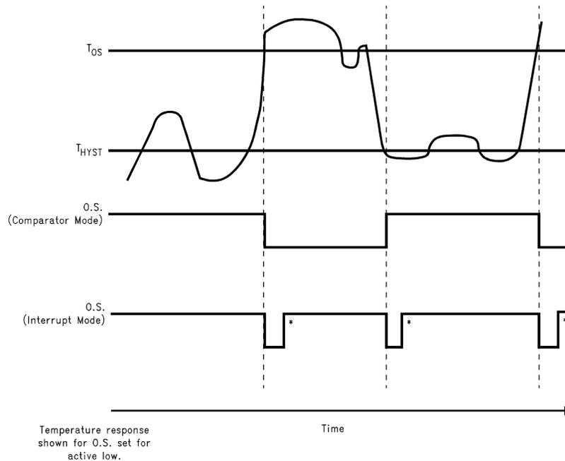
These interrupt mode resets of O.S. occur only when LM75 is read or placed in shutdown. Otherwise, O.S. would remain active indefinitely for any event.
