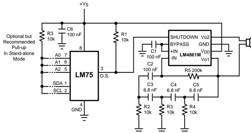
**Figure 15. Temperature Sensor with Loudmouth Alarm (Barking Watchdog)**
