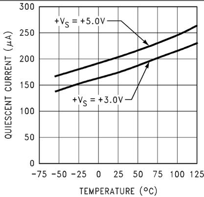
Figure 6. Static Quiescent Current vs Temperature (LM75C)
