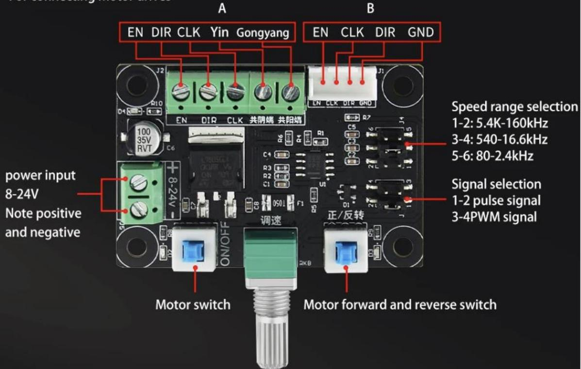
Different stepper motor drive port labels are not used but have the same function
