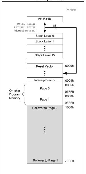
FIGURE 3-2: PROGRAM MEMORY MAP AND STACK FOR PIC16(L)F1509
