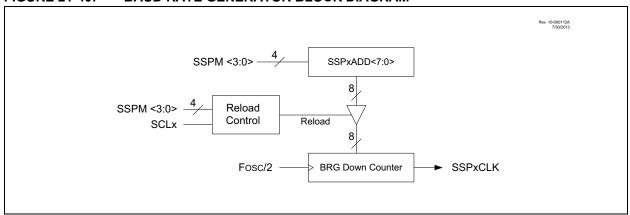
**Note:** Values of 0x00, 0x01 and 0x02 are not valid for SSPxADD when used as a Baud Rate Generator for I<sup>2</sup>C. This is an implementation limitation.
