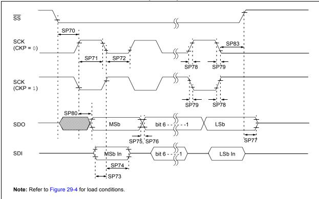
FIGURE 29-19: SPI SLAVE MODE TIMING (CKE = 1)
