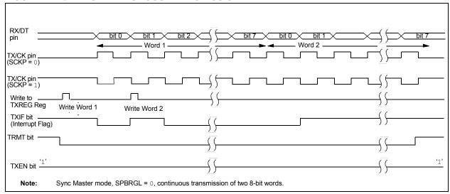
FIGURE 22-11: SYNCHRONOUS TRANSMISSION (THROUGH TXEN)
