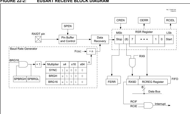
**FIGURE 22-2: EUSART RECEIVE BLOCK DIAGRAM**
