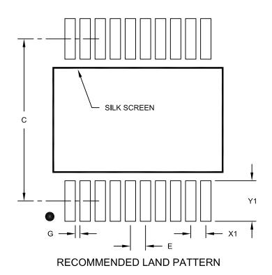
MILLIMETERS Units MIN MAX **Dimension Limits** NOM Contact Pitch 0.65 BSC Ε С Contact Pad Spacing 7.20 Contact Pad Width (X20) X1 0.45 Contact Pad Length (X20) <u>Y1</u> 1.75 Distance Between Pads G 0.20
