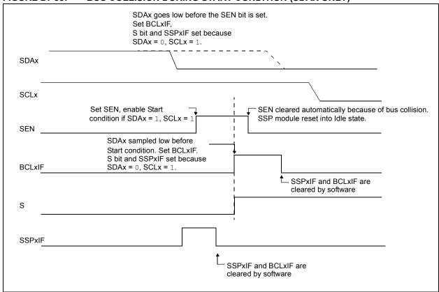
FIGURE 21-34: BUS COLLISION DURING START CONDITION (SCLX = 0)
