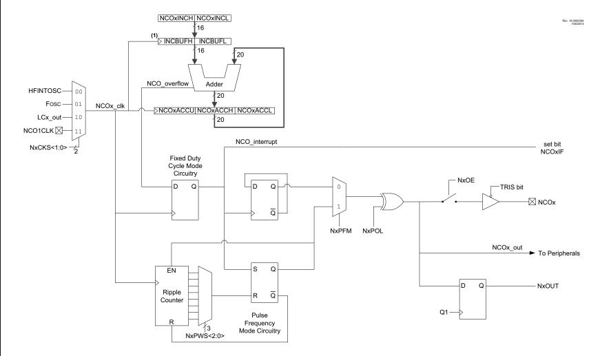
The increment registers are double-buffered to allow for value changes to be made without first disabling the NCO module. The full increment value is loaded into the buffer registers on the second rising edge of the NCOx clk signal that occurs immediately after a write to NCOxINCL register. The buffers are not user-accessible and are shown here for reference.
