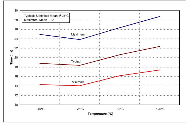
FIGURE 15-21: CVREF IPD vs. VDD OVER TEMPERATURE (HIGH RANGE)
