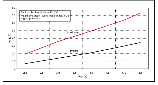
FIGURE 15-10: IDD vs. VDD (LP MODE)
