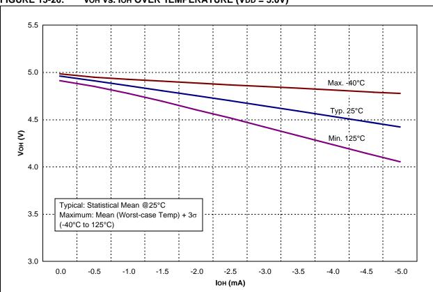
FIGURE 15-26: VOH vs. IOH OVER TEMPERATURE (VDD = 5.0V)
