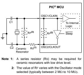
**3:** An additional parallel feedback resistor (RP) may be required for proper ceramic resonator operation.
