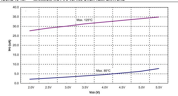
FIGURE 15-18: MAXIMUM WDT IPD vs. VDD OVER TEMPERATURE
