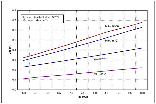
FIGURE 15-23: Vol vs. IoL OVER TEMPERATURE (VDD = 3.0V)
