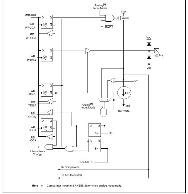
FIGURE 4-1: BLOCK DIAGRAM OF RA0
