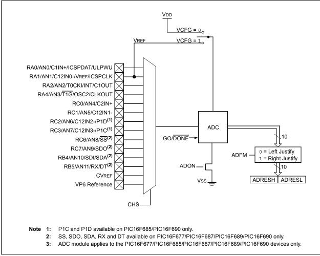
Figure 9-1 shows the block diagram of the ADC.
