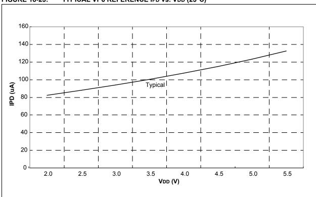
FIGURE 18-23: TYPICAL VP6 REFERENCE IPD vs. VDD (25°C)
