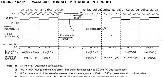
4: CLKOUT is not available in XT, HS, LP or EC Oscillator modes, but shown here for timing reference.
