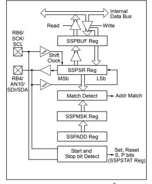
The SSP module has six registers for the  $I^2C$  operation, which are listed below.
