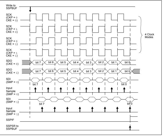
FIGURE 13-3: SPI MODE WAVEFORM (MASTER MODE)
