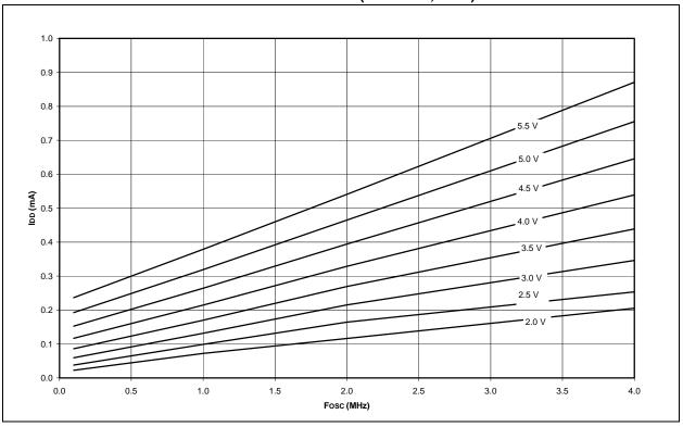
FIGURE 10-4: MAXIMUM IDD vs. Fosc OVER VDD (XT MODE, -40° TO +125°C)
