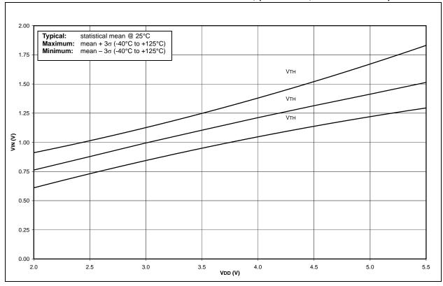
FIGURE 10-18: MINIMUM AND MAXIMUM VIN vs. VDD (ST INPUT, -40°C TO +125°C)
