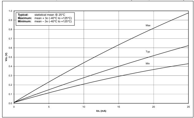
FIGURE 10-16: TYPICAL, MINIMUM AND MAXIMUM Vol vs. Iol (VDD = 3V, -40°C TO +125°C)
