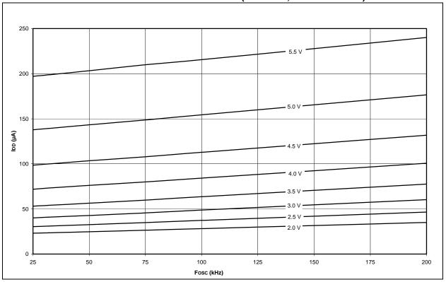
FIGURE 10-7: AVERAGE FOSC vs. VDD FOR R (RC MODE, C = 22 pF, 25°C)
