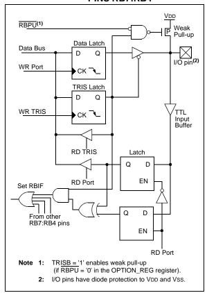
FIGURE 4-4: BLOCK DIAGRAM OF PINS RB3:RB0
