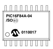
20-Lead SSOP (5.30 mm)
