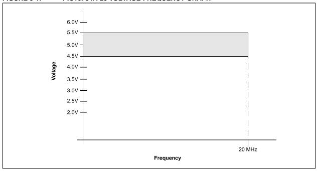
FIGURE 9-2: PIC16LF84A-04 VOLTAGE-FREQUENCY GRAPH
