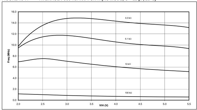
FIGURE 10-8: AVERAGE FOSC vs. VDD FOR R (RC MODE, C = 100 pF, 25°C)
