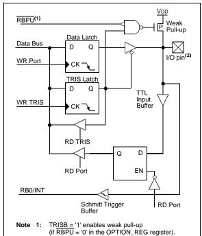
2: I/O pins have diode protection to VDD and Vss.
