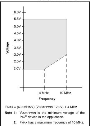
FIGURE 9-3: PIC16F84A-04 VOLTAGE-FREQUENCY GRAPH
