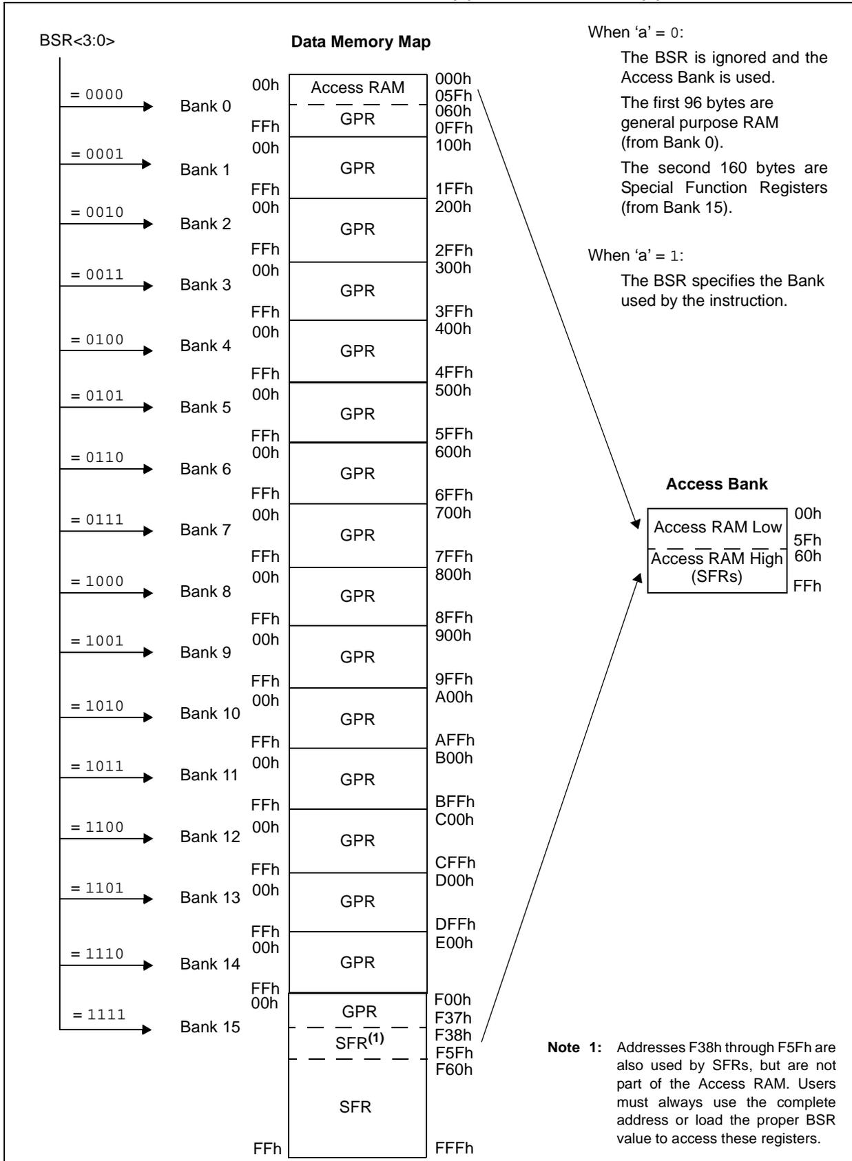
**FIGURE 5-9: USE OF THE BANK SELECT REGISTER (DIRECT ADDRESSING)**
