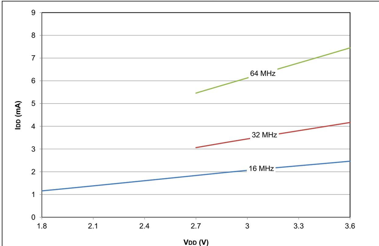
FIGURE 28-31: PIC18LF2X/4XK22 MAXIMUM  $I_{DD}$ : RC\_RUN HF-INTOSC with PLL
