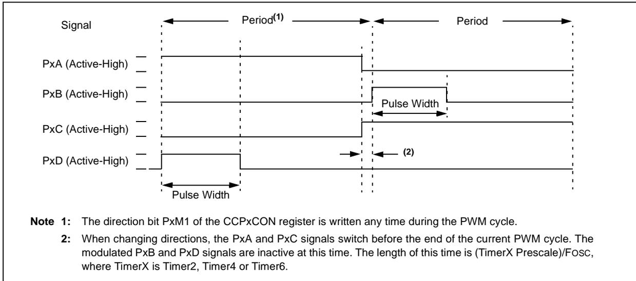
**FIGURE 14-13: EXAMPLE OF PWM DIRECTION CHANGE AT NEAR 100% DUTY CYCLE**
