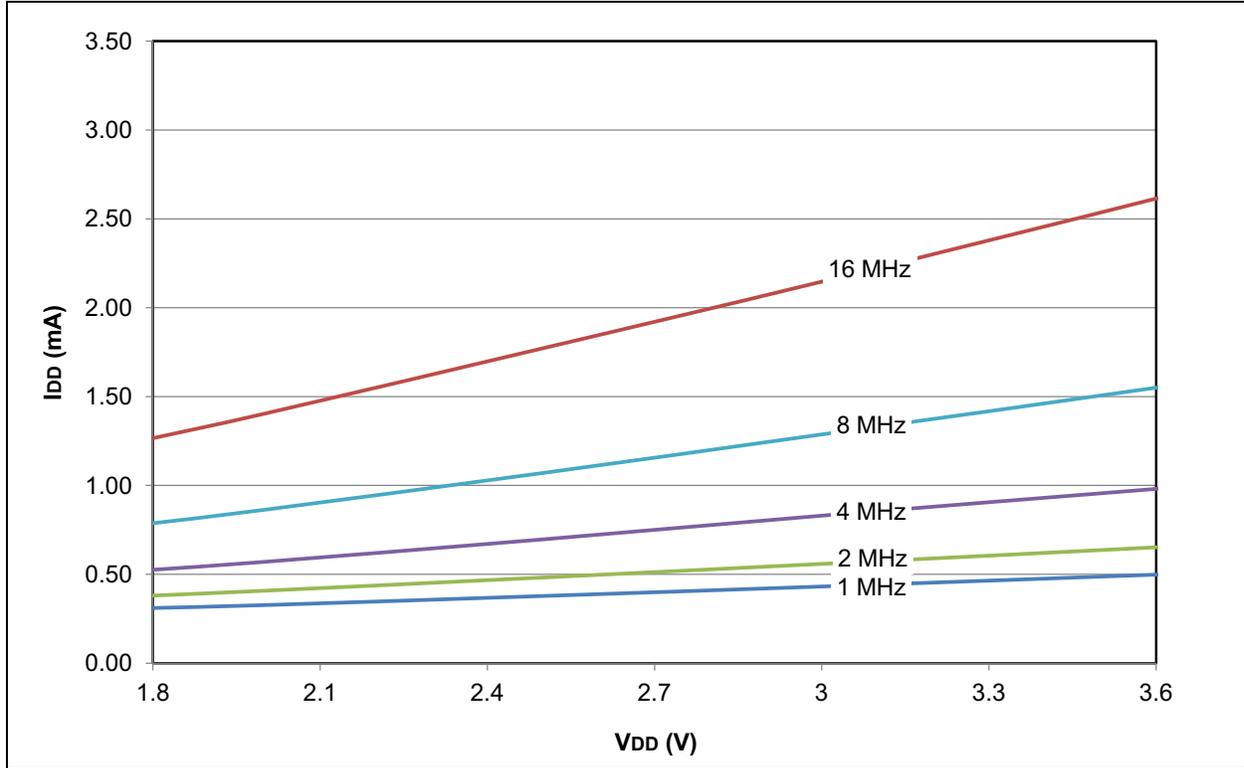
FIGURE 28-27: PIC18LF2X/4XK22 MAXIMUM  $I_{DD}$ : RC\_RUN HF-INTOSC
