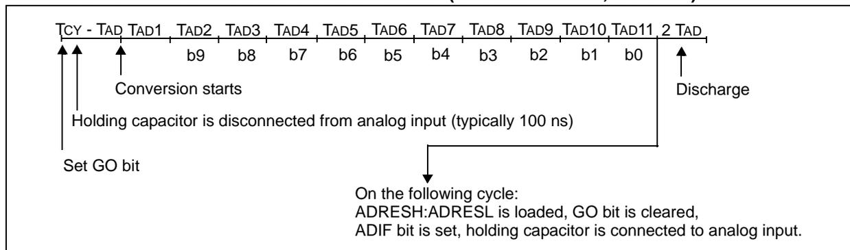
**FIGURE 17-4: A/D CONVERSION TAD CYCLES (ACQT<2:0> = 010, TACQ = 4 TAD)**
