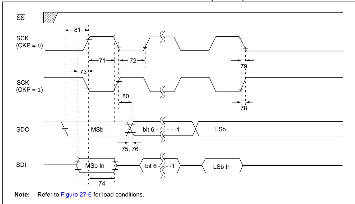
**FIGURE 27-15: EXAMPLE SPI SLAVE MODE TIMING (CKE = 0)**
