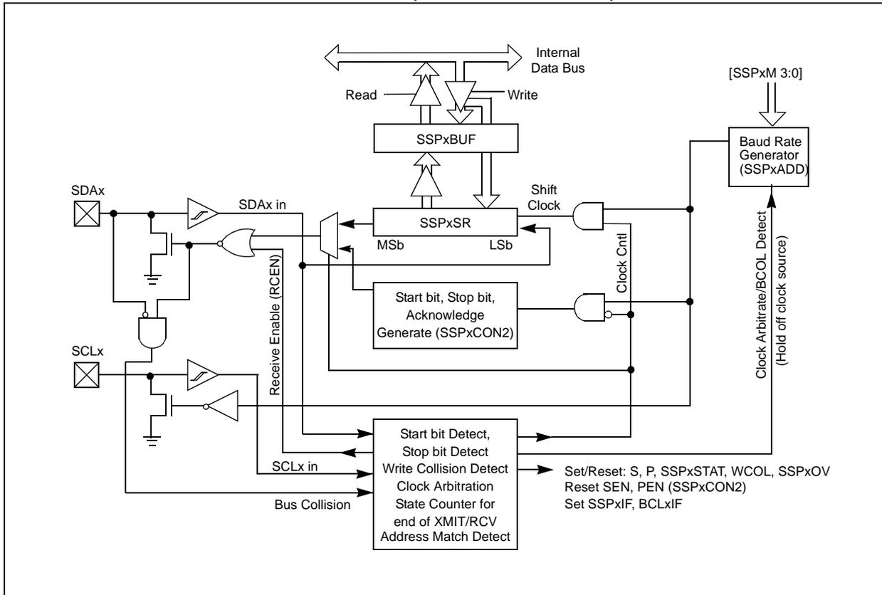
**FIGURE 15-3: MSSPx BLOCK DIAGRAM (I<sup>2</sup>C™ SLAVE MODE)**
