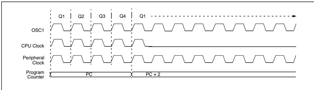
**FIGURE 3-7: TRANSITION TIMING FOR WAKE FROM IDLE TO RUN MODE**
