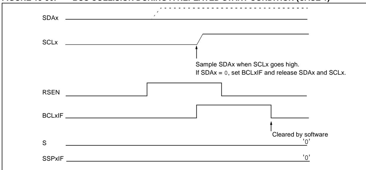
**FIGURE 15-37: BUS COLLISION DURING REPEATED START CONDITION (CASE 2)**
