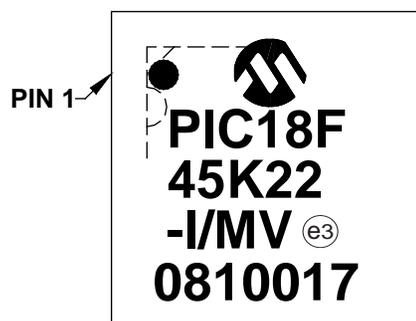
44-Lead QFN (8x8x0.9 mm)
