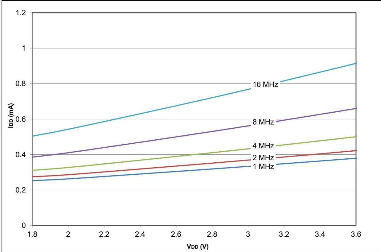
FIGURE 28-41: PIC18LF2X/4XK22 MAXIMUM  $I_{DD}$ : RC\_IDLE HF-INTOSC
