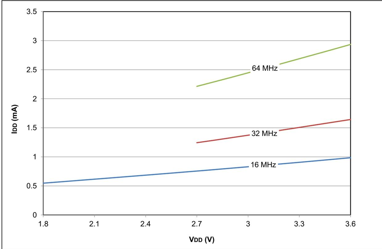
FIGURE 28-45: PIC18LF2X/4XK22 MAXIMUM  $I_{DD}$ : RC\_IDLE HF-INTOSC with PLL
