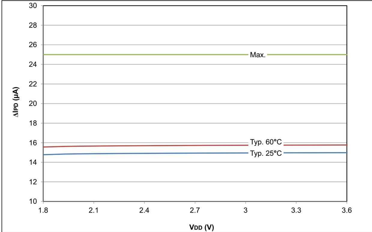
FIGURE 28-18: PIC18F2X/4XK22 DELTA I<sub>PD</sub> FVR
