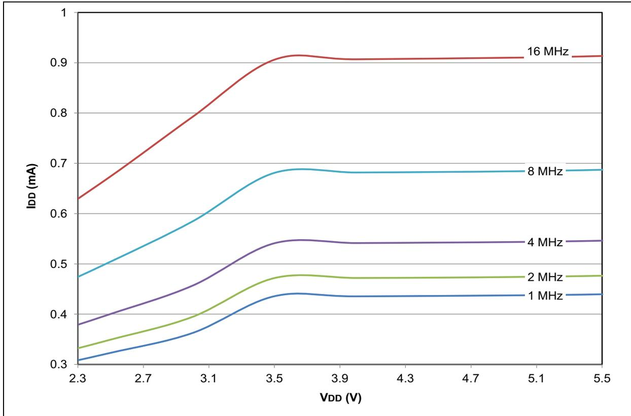
FIGURE 28-43: PIC18F2X/4XK22 MAXIMUM  $I_{DD}$ : RC\_IDLE HF-INTOSC
