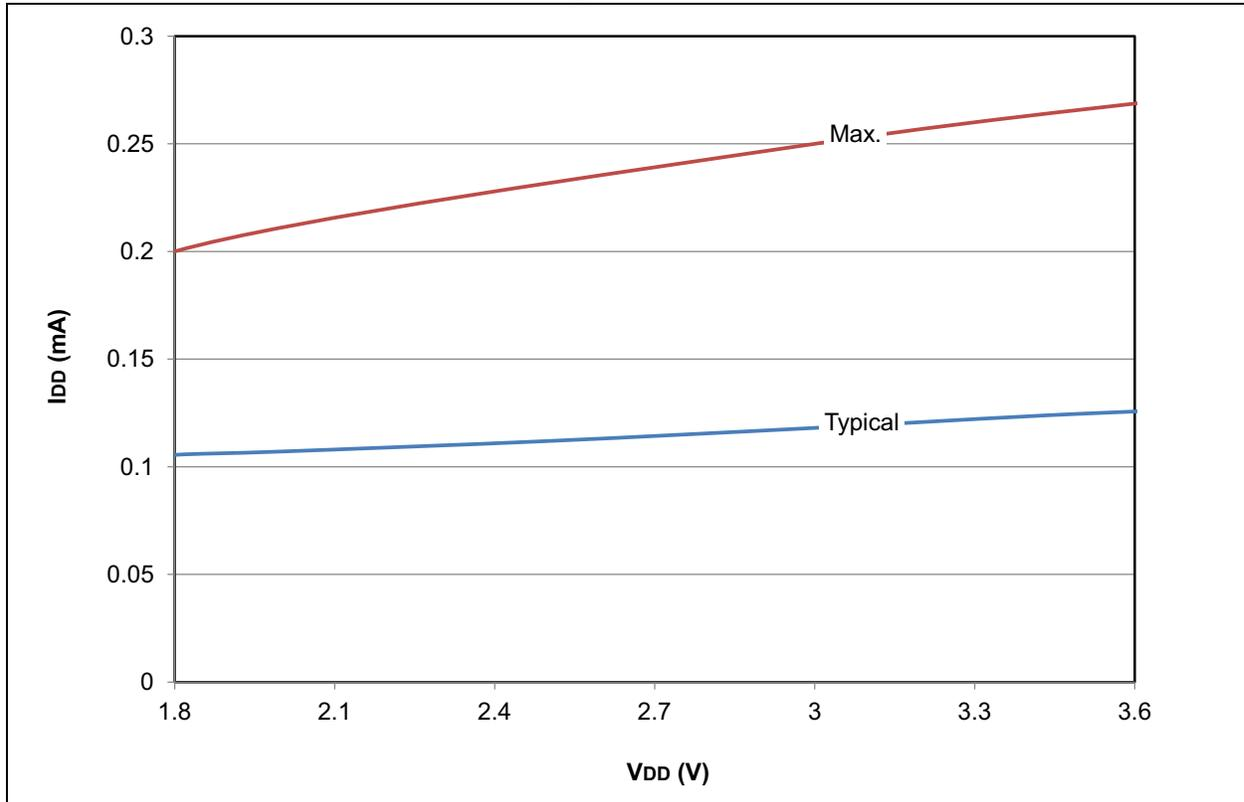
FIGURE 28-39: PIC18F2X/4XK22 I<sub>DD</sub>: RC\_IDLE MF-INTOSC 500 kHz
