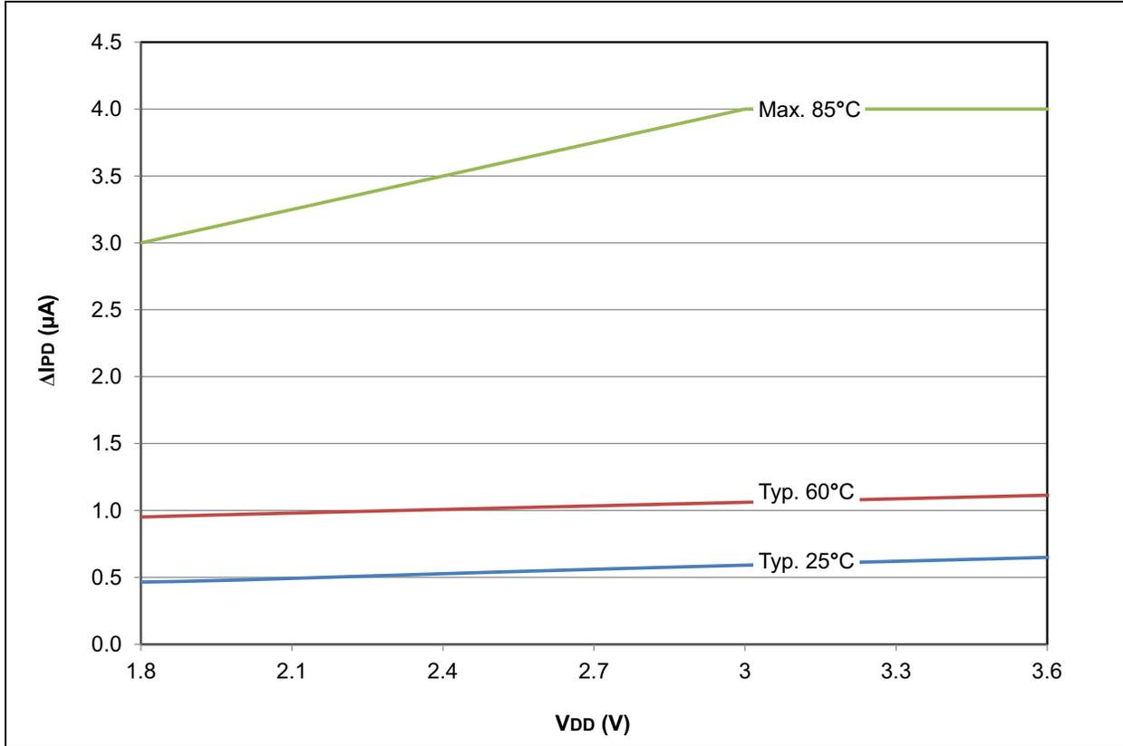
FIGURE 28-10: PIC18F2X/4XK22 DELTA I<sub>PD</sub> SECONDARY OSCILLATOR
