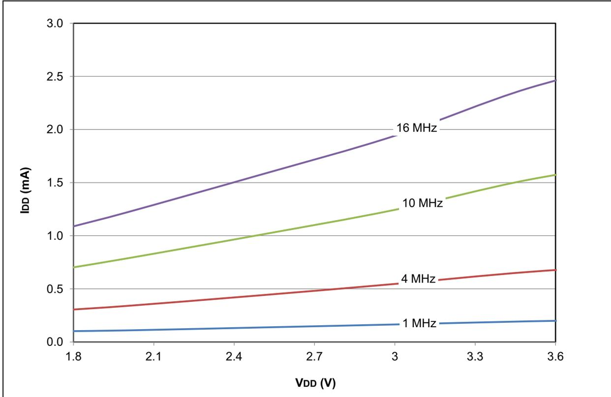
FIGURE 28-49: PIC18LF2X/4XK22 MAXIMUM  $I_{DD}$ : PRI\_RUN EC MEDIUM POWER
