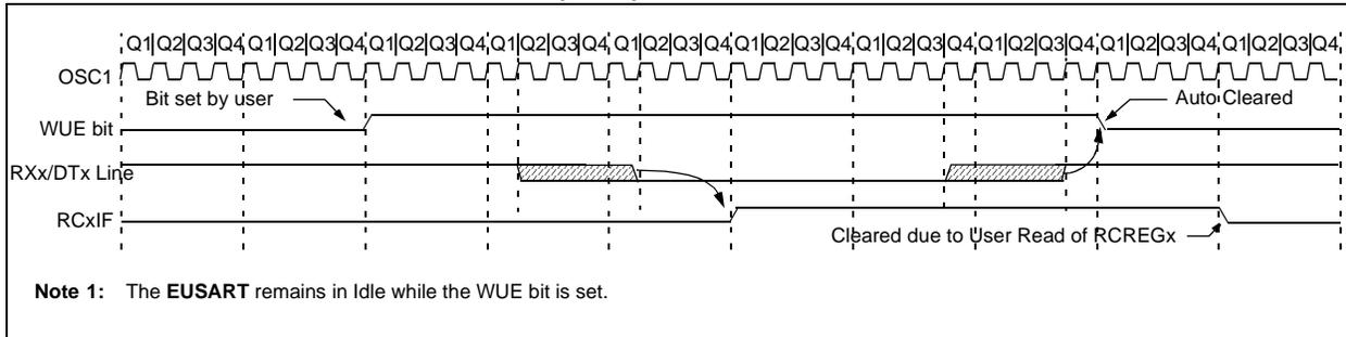
**FIGURE 16-8: AUTO-WAKE-UP BIT (WUE) TIMINGS DURING SLEEP**
