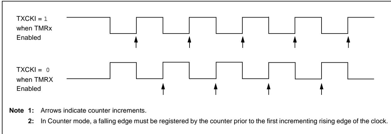
**FIGURE 12-4: TIMER1/3/5 GATE ENABLE MODE**
