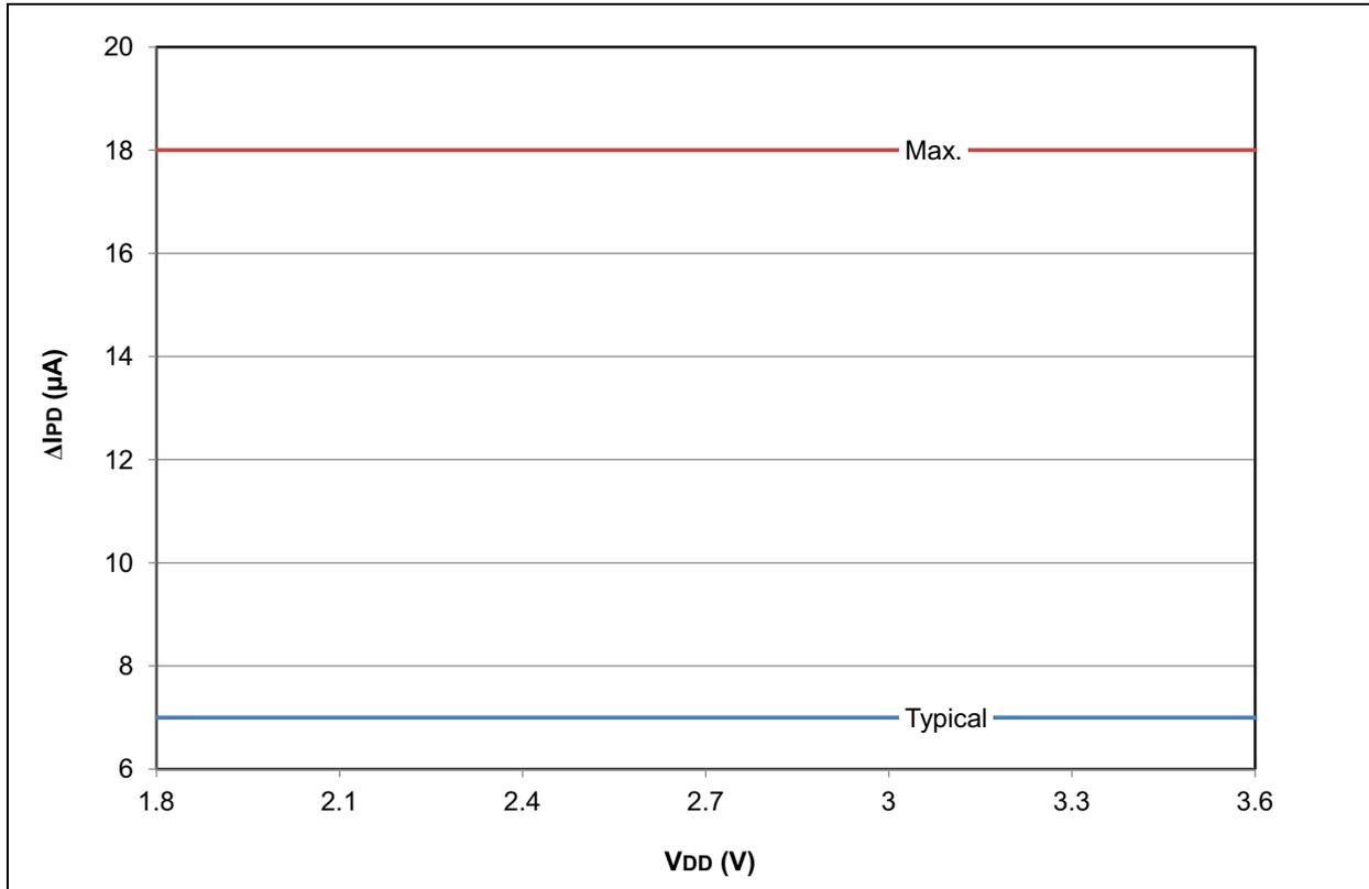
FIGURE 28-12: PIC18F2X/4XK22 DELTA I<sub>PD</sub> COMPARATOR LOW-POWER MODE
