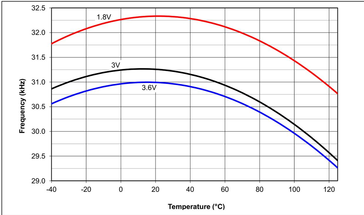
**FIGURE 28-104: PIC18F2X/4XK22 TYPICAL LF-INTOSC FREQUENCY vs. TEMPERATURE**
