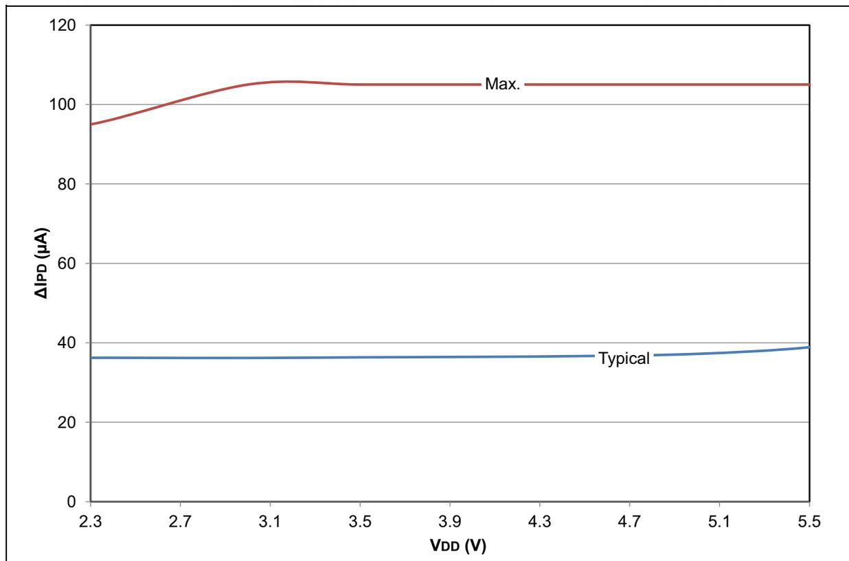
FIGURE 28-15: PIC18LF2X/4XK22 DELTA I<sub>PD</sub> DAC
