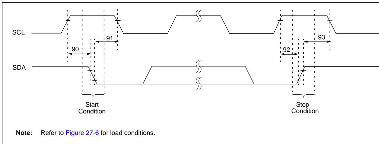
**TABLE 27-18: MASTER SSP I<sup>2</sup>C™ BUS START/STOP BITS REQUIREMENTS**
