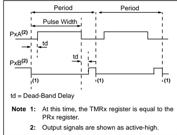
**FIGURE 14-9: EXAMPLE OF HALF-BRIDGE APPLICATIONS**
