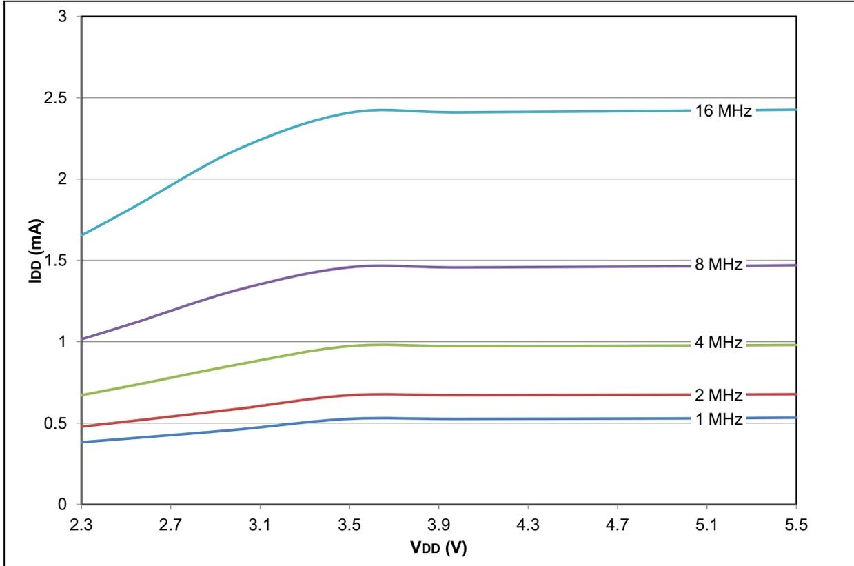
FIGURE 28-29: PIC18F2X/4XK22 MAXIMUM  $I_{DD}$ : RC\_RUN HF-INTOSC
