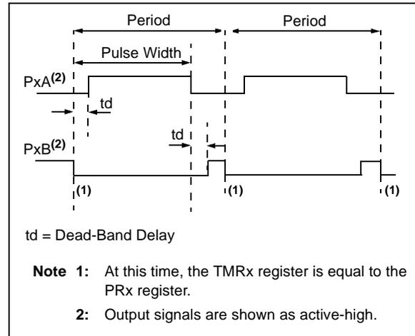
**FIGURE 14-17: EXAMPLE OF HALF-BRIDGE APPLICATIONS**
