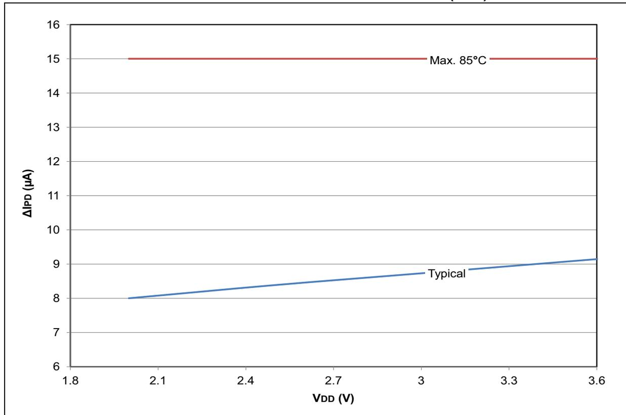
FIGURE 28-6: PIC18F2X/4XK22 DELTA I<sub>PD</sub> BROWN-OUT RESET (BOR)
