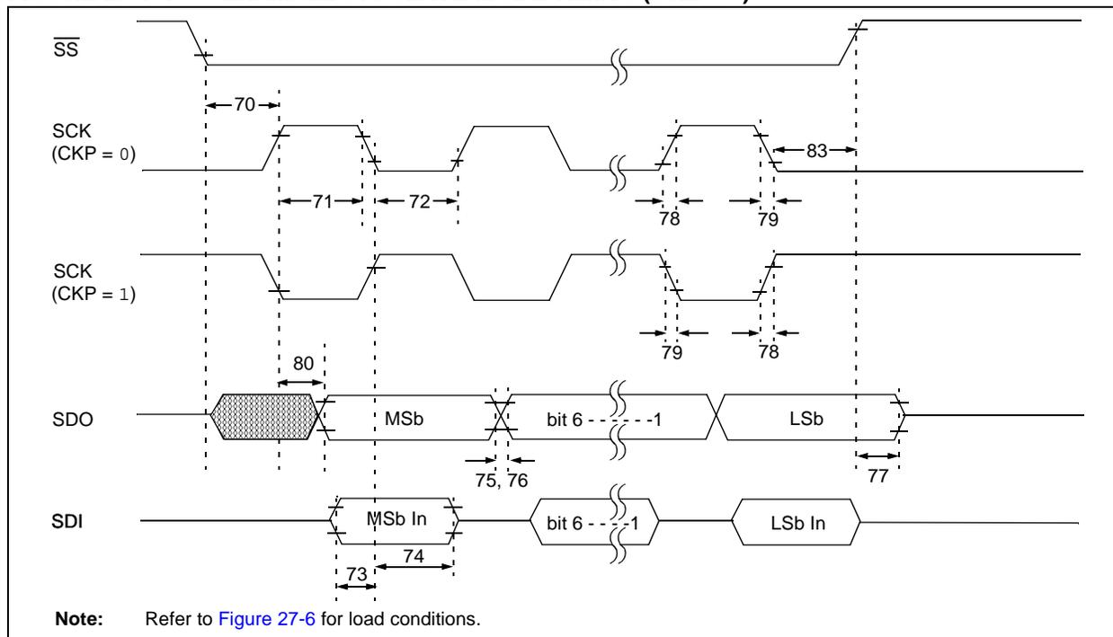
**TABLE 27-15: EXAMPLE SPI MODE REQUIREMENTS (SLAVE MODE TIMING, CKE = 0 OR 1)**
