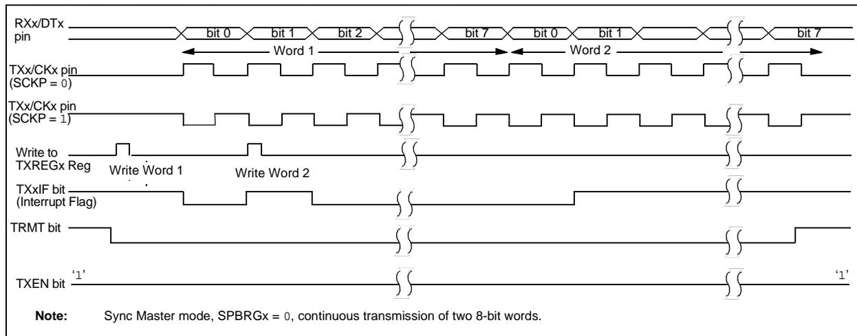
**FIGURE 16-11: SYNCHRONOUS TRANSMISSION (THROUGH TXEN)**
