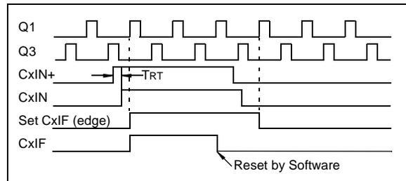
**FIGURE 18-4: COMPARATOR INTERRUPT TIMING WITH CMxCON0 READ**
