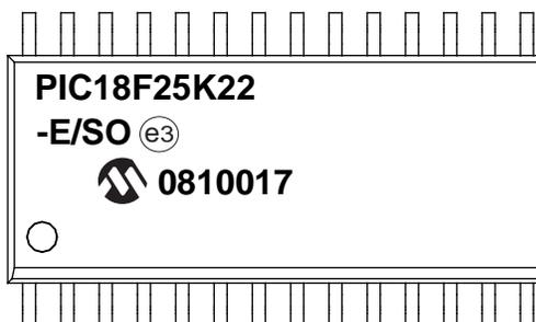
28-Lead SSOP (5.30 mm)
