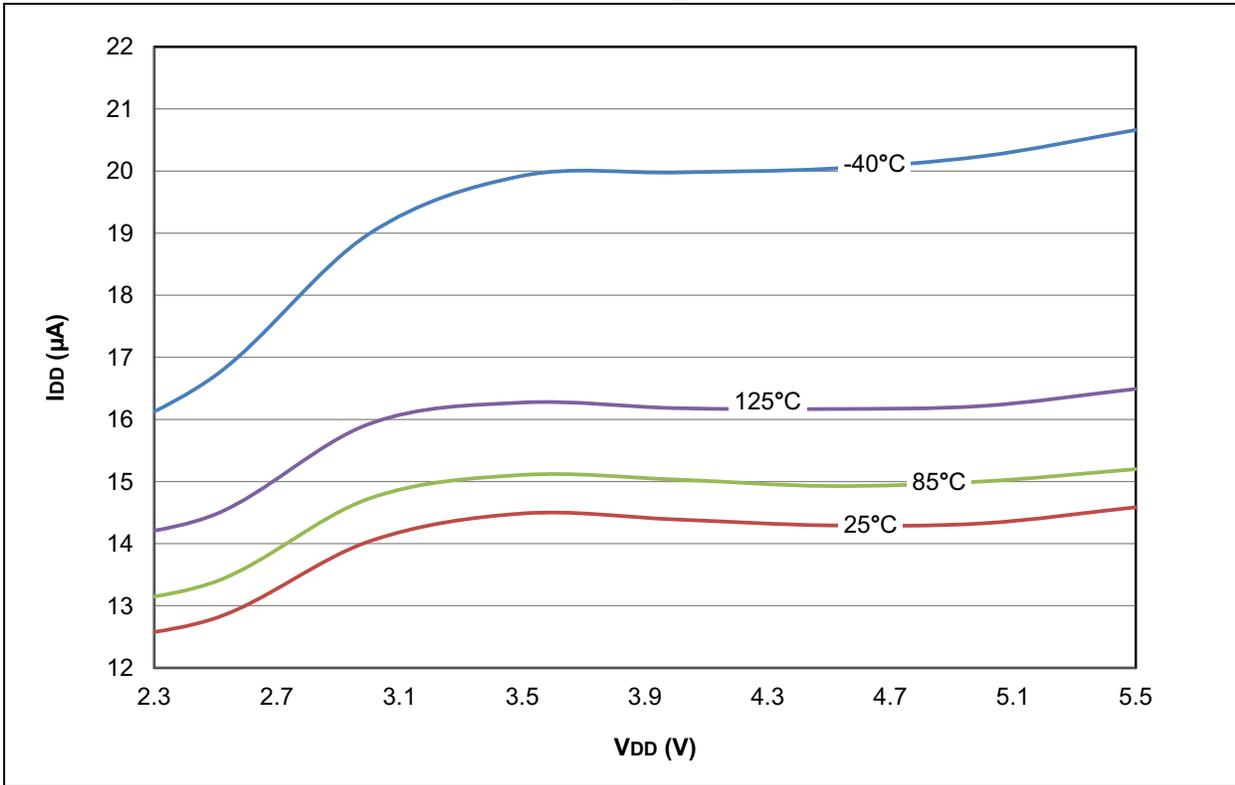
FIGURE 28-37: PIC18F2X/4XK22 MAXIMUM  $I_{DD}$ : RC\_IDLE LF-INTOSC 31 kHz
