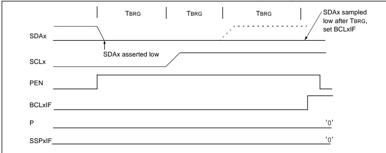
**FIGURE 15-39: BUS COLLISION DURING A STOP CONDITION (CASE 2)**
