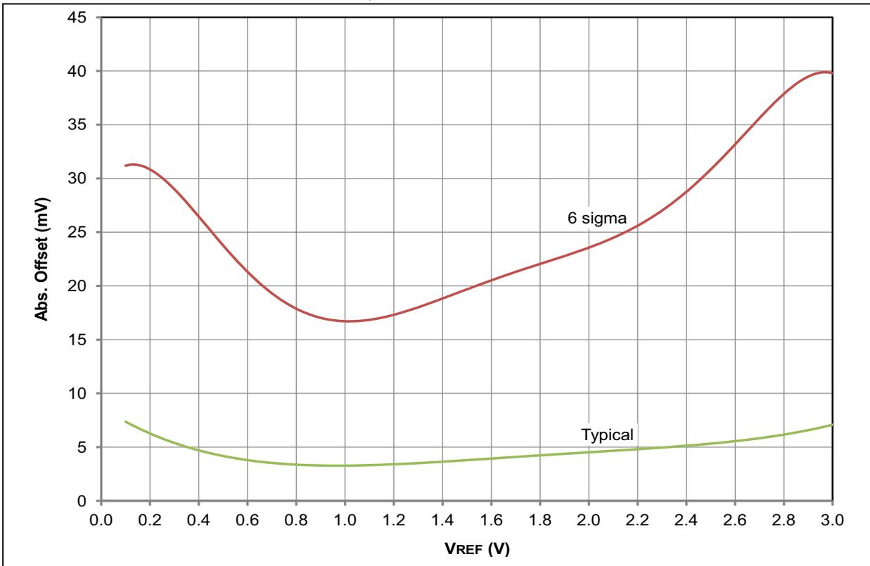
**FIGURE 28-89: PIC18LF2X/4XK22 COMPARATOR OFFSET VOLTAGE, NORMAL-POWER MODE;  $V_{DD}=1.8V$**
