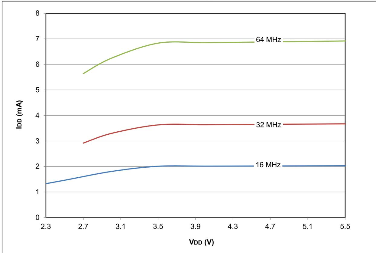
FIGURE 28-59: PIC18F2X/4XK22 MAXIMUM  $I_{DD}$ : PRI\_RUN EC with PLL
