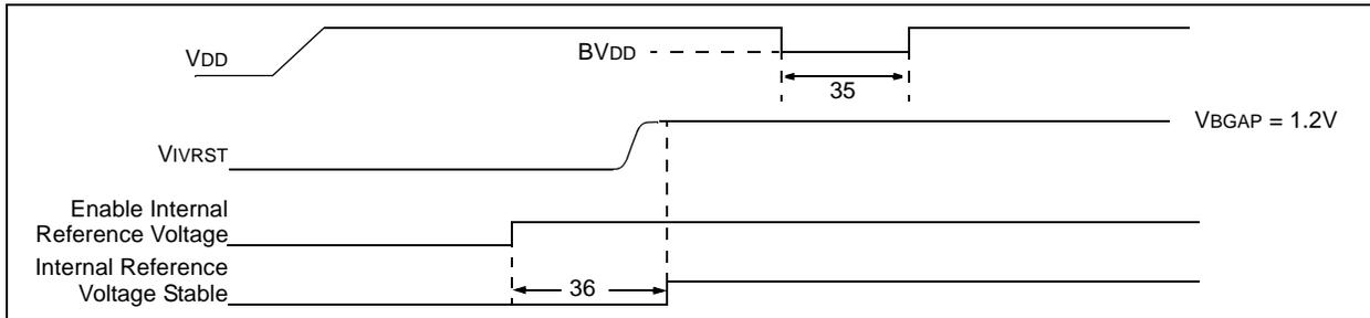
**TABLE 27-11: RESET, WATCHDOG TIMER, OSCILLATOR START-UP TIMER, POWER-UP TIMER AND BROWN-OUT RESET REQUIREMENTS**
