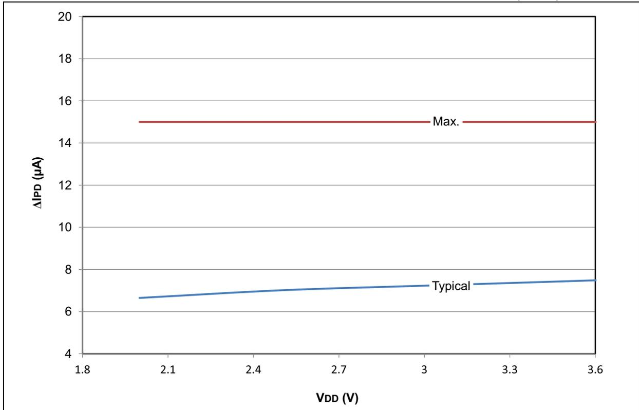
FIGURE 28-8: PIC18F2X/4XK22 DELTA I<sub>PD</sub> HIGH/LOW-VOLTAGE DETECT (HLVD)
