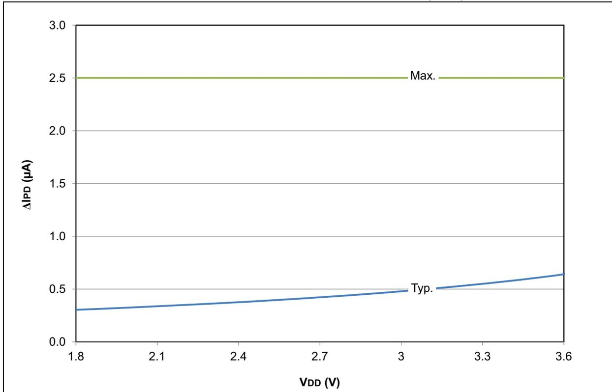
**FIGURE 28-4: PIC18F2X/4XK22 DELTA I<sub>PD</sub> WATCHDOG TIMER (WDT)**
