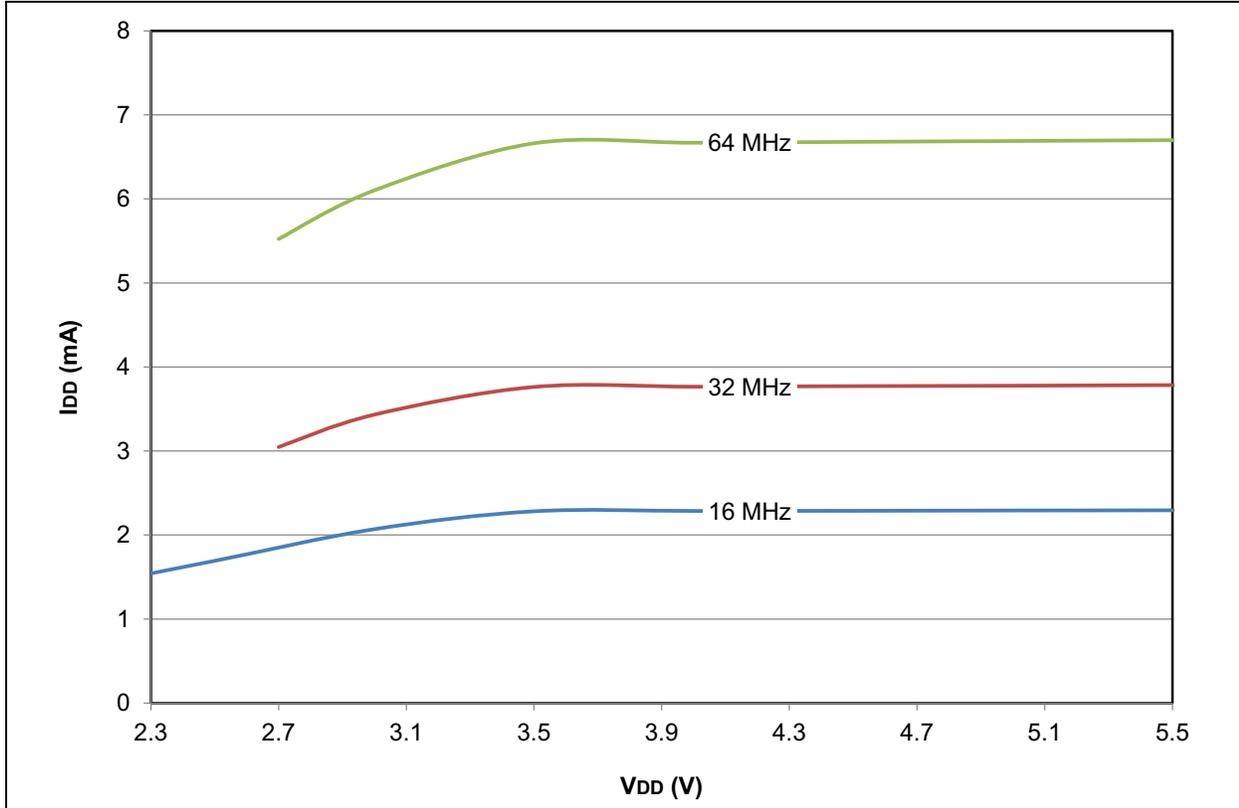
FIGURE 28-33: PIC18F2X/4XK22 MAXIMUM  $I_{DD}$ : RC\_RUN HF-INTOSC with PLL
