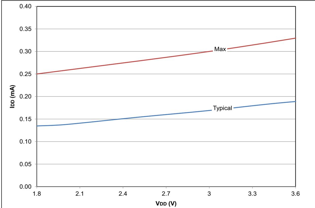
FIGURE 28-25: PIC18F2X/4XK22 I<sub>DD</sub>: RC\_RUN MF-INTOSC 500 kHz
