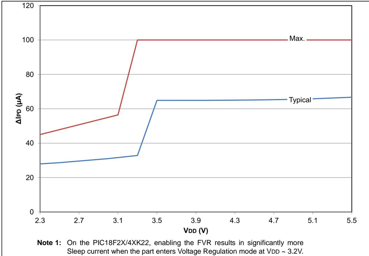
FIGURE 28-19: PIC18(L)F2X/4XK22 DELTA I<sub>DD</sub> A/D CONVERTOR<sup>1</sup>
