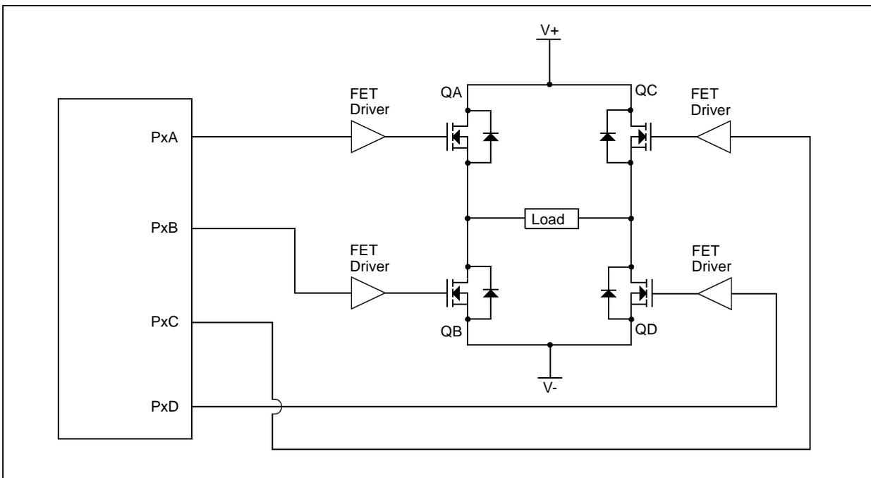
**FIGURE 14-11: EXAMPLE OF FULL-BRIDGE PWM OUTPUT**
