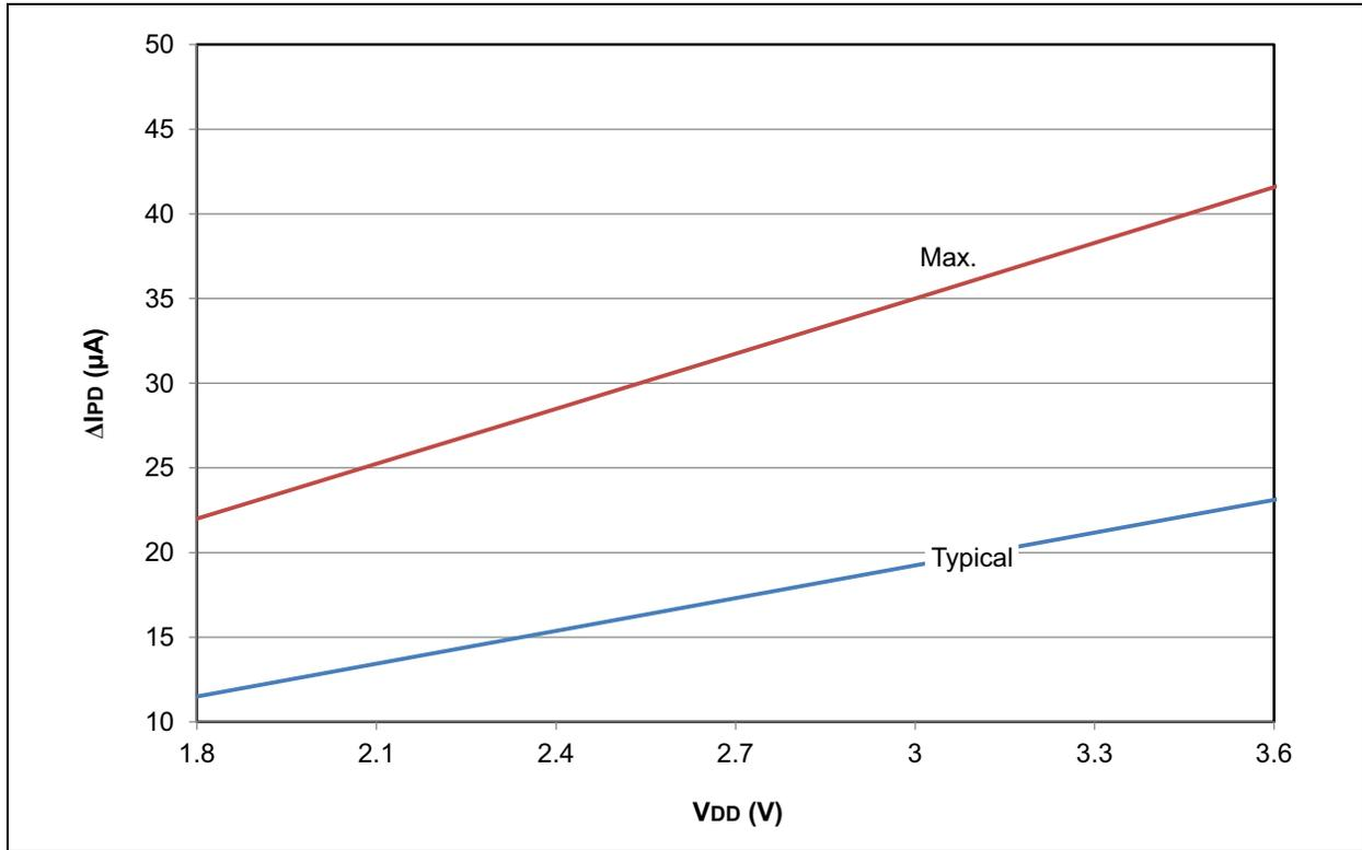
FIGURE 28-16: PIC18F2X/4XK22 DELTA I<sub>PD</sub> DAC
