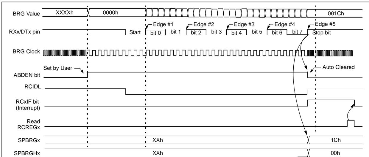
**Note 1:** The ABD sequence requires the EUSART module to be configured in Asynchronous mode.
