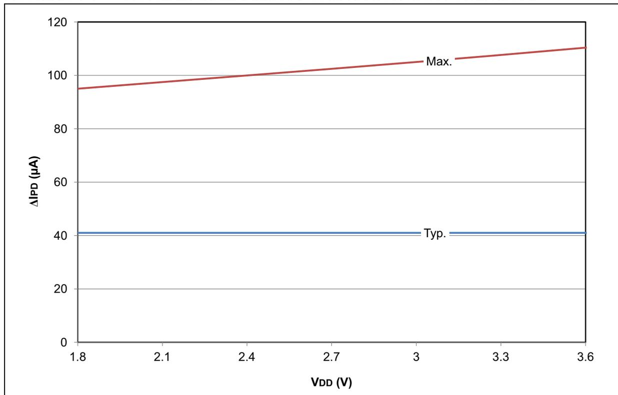
FIGURE 28-14: PIC18F2X/4XK22 DELTA IPD COMPARATOR HIGH-POWER MODE
