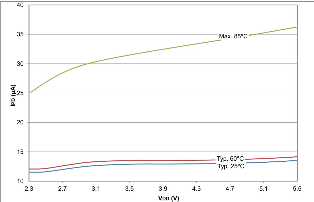
**FIGURE 28-3: PIC18LF2X/4XK22 DELTA I<sub>PD</sub> WATCHDOG TIMER (WDT)**
