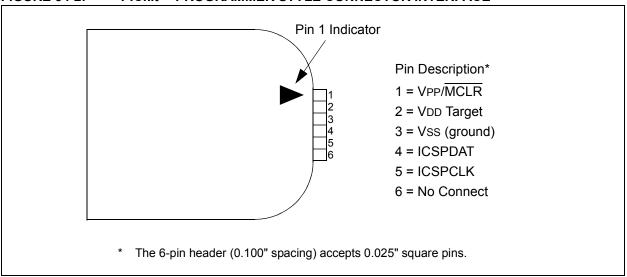
FIGURE 34-3: TYPICAL CONNECTION FOR ICSP™ PROGRAMMING
