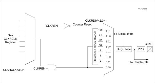
FIGURE 5-2: CLOCK REFERENCE TIMING
