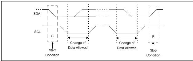
FIGURE 26-13: I<sup>2</sup>C RESTART CONDITION
