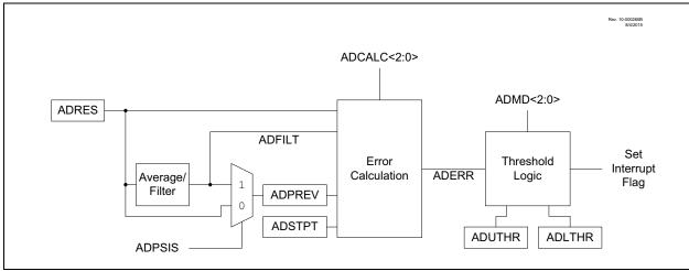
The operation of the ADC computational features is controlled by ADMD <2:0> bits in the ADCON2 register.
