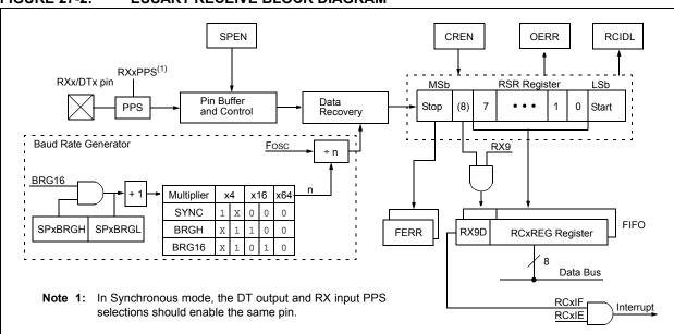
FIGURE 27-2: EUSART RECEIVE BLOCK DIAGRAM
