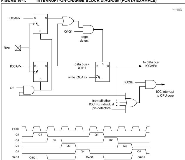
**FIGURE 16-1:** INTERRUPT-ON-CHANGE BLOCK DIAGRAM (PORTA EXAMPLE)
