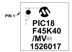
44-Lead QFN (8x8x0.9 mm)
