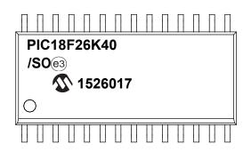
28-Lead SSOP (5.30 mm)
