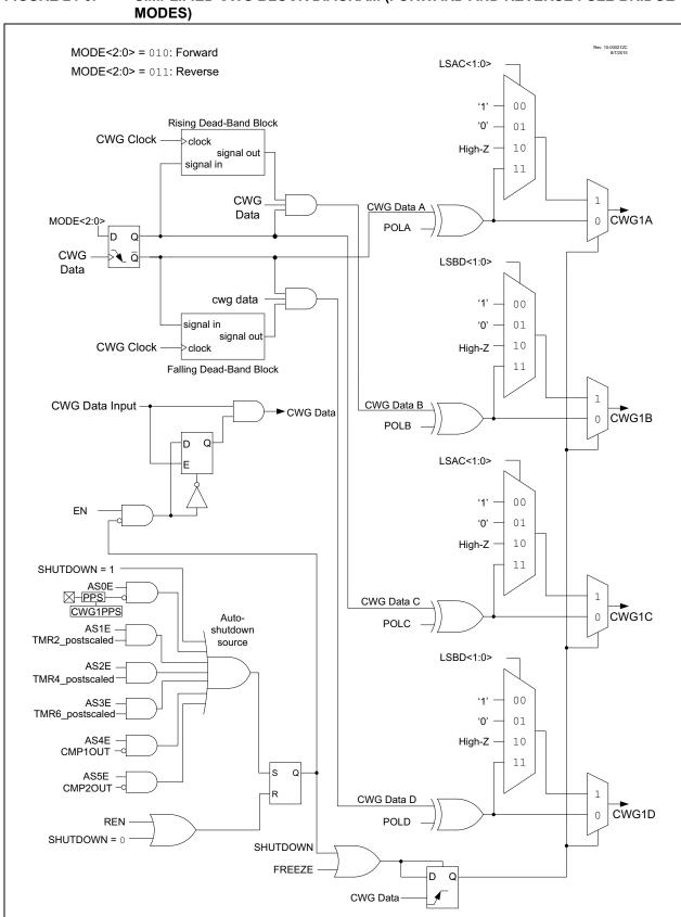
**FIGURE 24-6:** SIMPLIFIED CWG BLOCK DIAGRAM (FORWARD AND REVERSE FULL-BRIDGE
