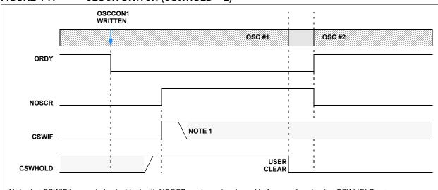
Note 1: CSWIF is asserted coincident with NOSCR, and may be cleared before or after clearing CSWHOLD = 0.
