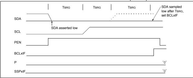
FIGURE 26-39: BUS COLLISION DURING A STOP CONDITION (CASE 2)
