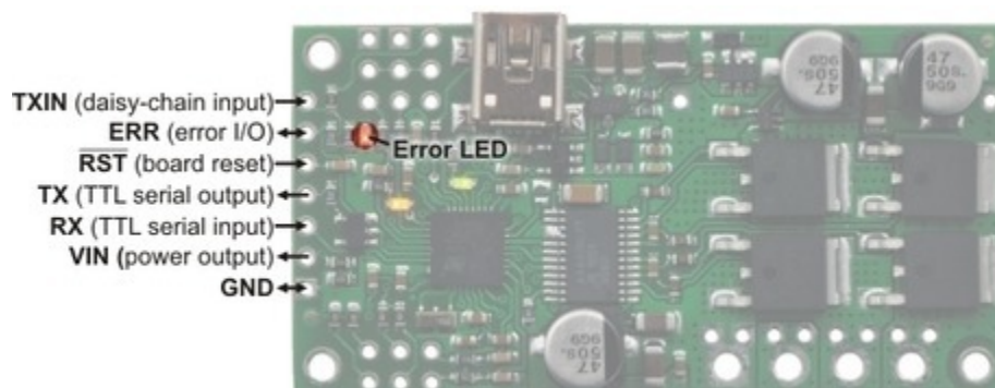
Simple High-Power Motor Controller 18v25 or 24v23 serial connections.
