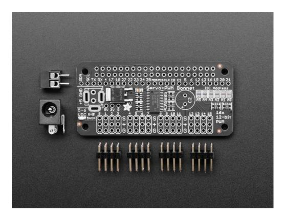
The Adafruit 16-Channel 12-bit PWM/Servo HAT or Bonnet will drive up to 16 servos or PWM outputs over I2C with only 2 pins. The on-board PWM controller will drive all 16 channels simultaneously with no additional Raspberry Pi processing overhead. What's more, you can stack up to 62 of them to control up to 992 servos - all with the same 2 pins!
