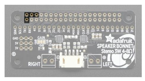
The two amplifier chips use the 3V + 5V + GND power pin at the 'top' of the 2x20 header. If using 3W speakers, you can draw a significant amount of current, over 1.5 Amps! Make sure you power your Pi with a good wall adapter like our 2.4A microUSB power plug.
