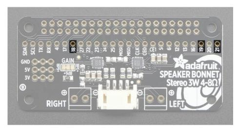
The Bonnet uses 3 data pins and they cannot be changed! Pins #18, #19 and #21 are used. All other pins are available
