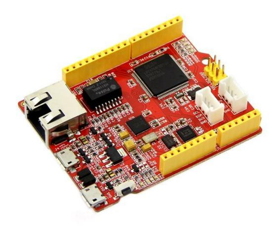
Arch Pro is an mbed enabled development board for rapid prototyping. It is a variant of mbed LPC1768 with built-in Ethernet, USB Host/Device, Grove connectors and Arduino form factor. With a variety of Shield and Grove modules and lots of software libraries for Arch Pro, you can implement Ethernet, USB Host/Device and NFC applications rapidly and easily.
