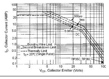
There are two limitations on the power handling ability of a transistor: average junction temperature and second breakdown safe operating area curves indicate  $I_{\rm C}\text{-}V_{\rm CE}$  limits of the transistor that must be observed for reliable operation i.e., the transistor must not be subjected to greater dissipation than the curves indicate.
