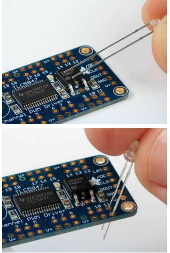
Connecting Monochrome LEDs Note that one leg of the led is longer than the other. This is the Anode and should be connected to the V+ hole in the board.
