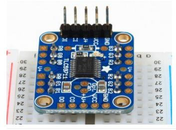
Repeat for the other side Flip the board over and repeat the process for the LED headers on the bottom of the board.
