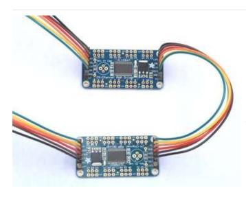
Multiple boards can be chained to control hundreds of LEDs. Using an Arduino, you will run out of memory long before you exceed the chaining capacity of these boards!
