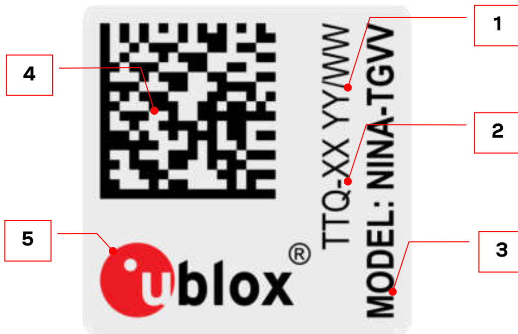
Figure 11: Location of product type number on the NINA-W10 series module label
