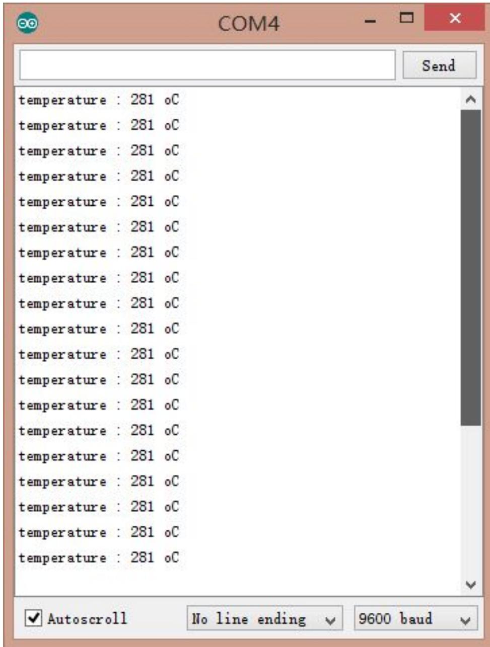
**NOTE:** This temperature was magnified 10 times, in the test, actual temperature is 28.1 degrees Celsius.
