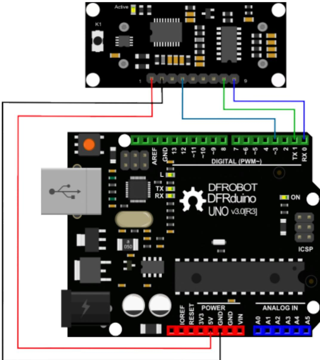
Download the sample code to the Arduino board, then wire as shown modules and Arduino connected on ultrasonic distance measurement can be achieved. **Note:**download first before connect the Arduino TX/RX, or download will failed.
