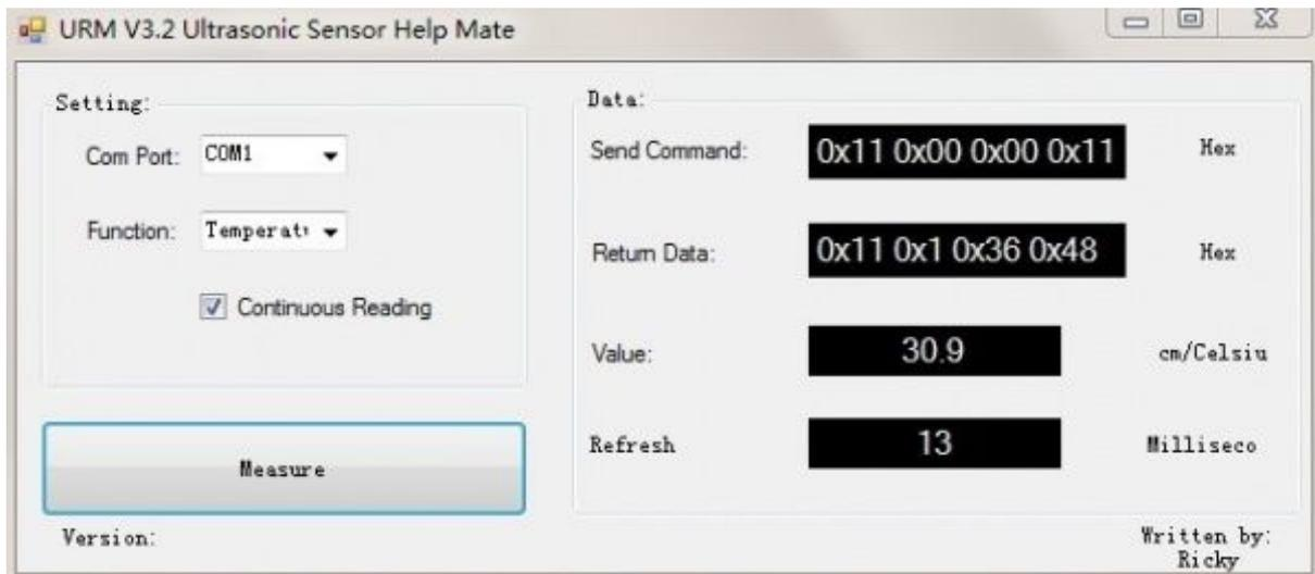
The usage of the software is very simple: ensure that there is no other software on the computer occupied the serial port, and then run Mate.exe, select the COM Port, and choose the parameter what you want to measure, and choose the "Continuous Reading ". Click "Measure" it will measure the temperature and the distance.
