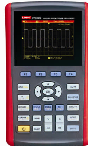
Figure 3-3 UTD1000L Series Front Panel
