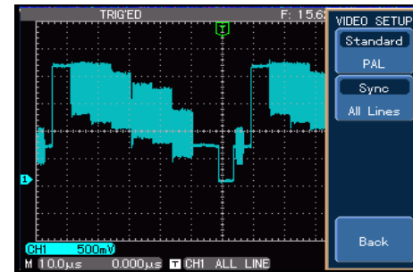
Figure 2-16 Video trigger : Line synchronization
