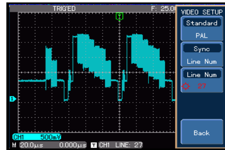
Figure 3-11 Video line triggering
