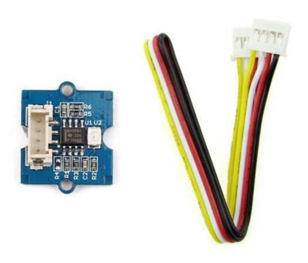
The Grove – UV Sensor is used for detecting the intensity of incident ultraviolet(UV) radiation. This form of electromagnetic radiation has shorter wavelengths than visible radiation. The Grove - UV Sensor is based on the sensor GUVA-S12D which has a wide spectral range of 200nm-400nm. The module outputs electrical signal which varies with the UV intensity, which gives your suggestion if it is a good idea to beach today.
