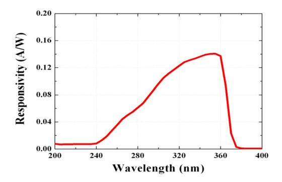
About our Grove - UV Sensor, we have converted Photocurrent to corresponding voltage value collected by Arduino/Seeeduino. The output voltage and the UV index is linear:
